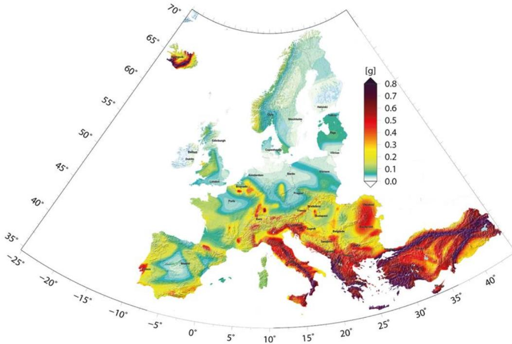
**Figure S13.** Peak Ground Acceleration (PGA) exceedance probabilities of 2 % in 50 years (average return period of 2475 years, reference rock velocity of  $v_s = 800$  m/s) [65].
