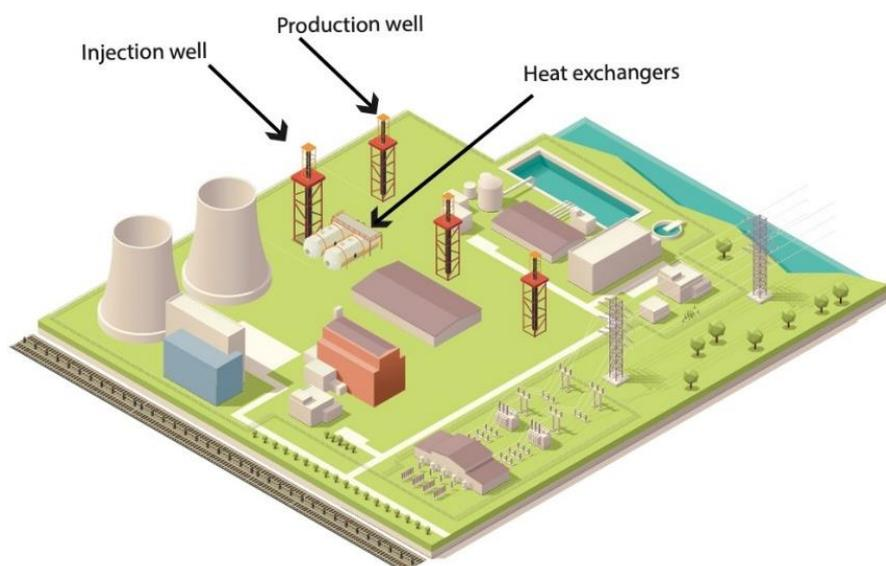
**Figure S12.** Coal plant converted to an enhanced geothermal system plant.
