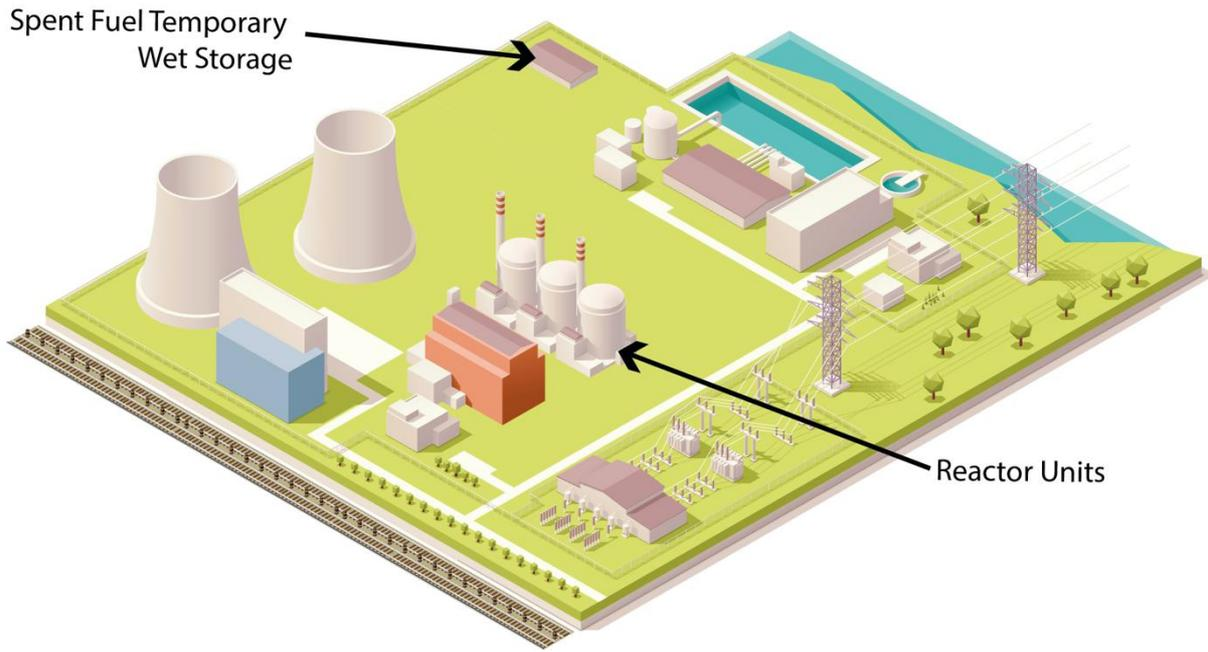
**Figure S19.** Step 3. Finished retrofit decarbonized coal site.
