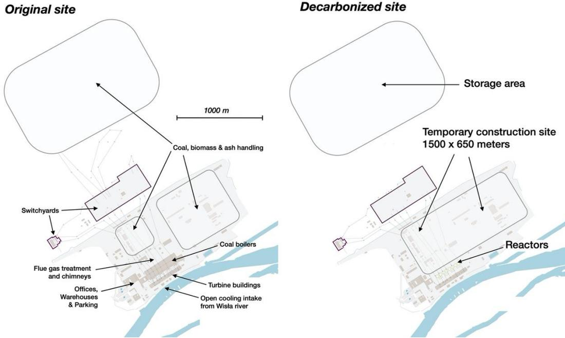
Figure S22. Retrofit decarbonization of Połaniec with nuclear reactors.
