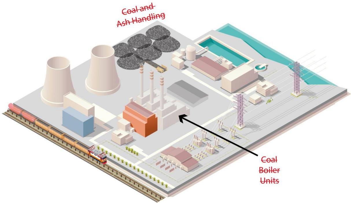
Figure S17. Step 1: Decommissioning coal-related on-site equipment.
