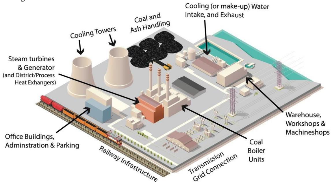
Figure S1. Coal Power Plant Site Layout and Major Components.
