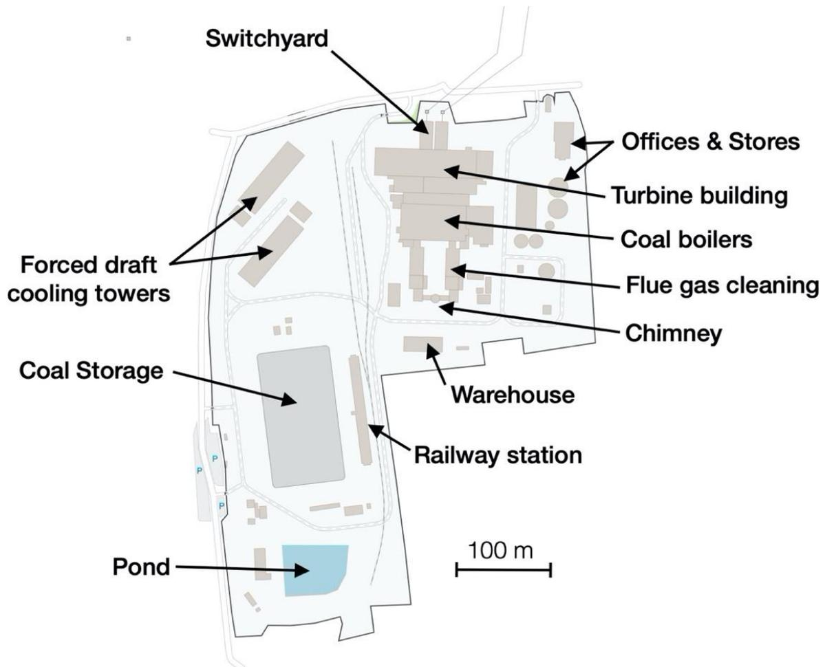
**Figure S5.** The Chorzów CHP plant layout (based on OpenStreetMap layers).
