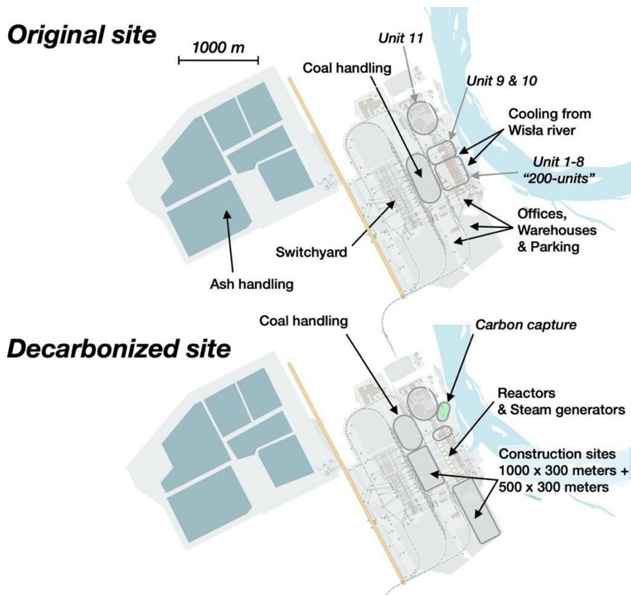
**Figure S21.** Retrofit decarbonization of Kozienice with nuclear reactors and carbon capture.
