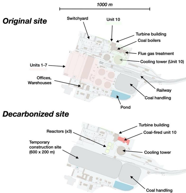
**Figure S20.** Retrofit decarbonization of Łagisza unit B10 with 3xKP-FHR, while unit remains in operation.
