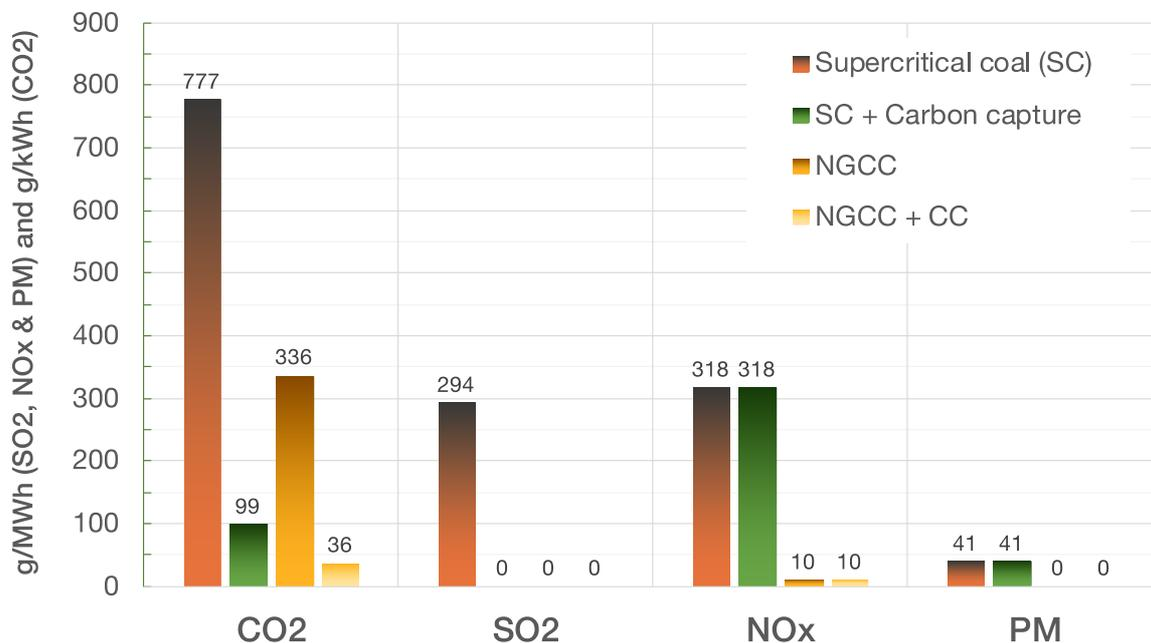
**Figure S2.** Air pollution impacts of adding carbon capture by NETL (developed from ref. [4])
