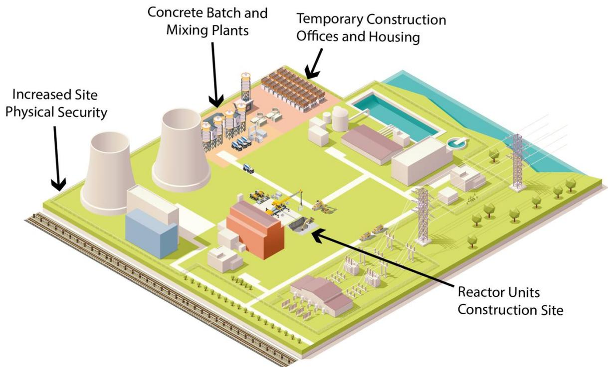
Figure S18. Step 2: Establishing nuclear reactor building construction site.
