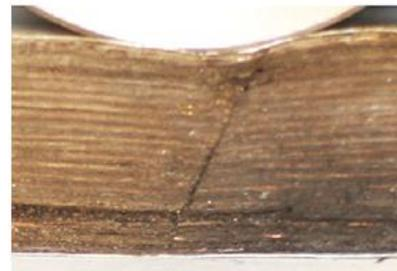
Failure mode of jelly roll
