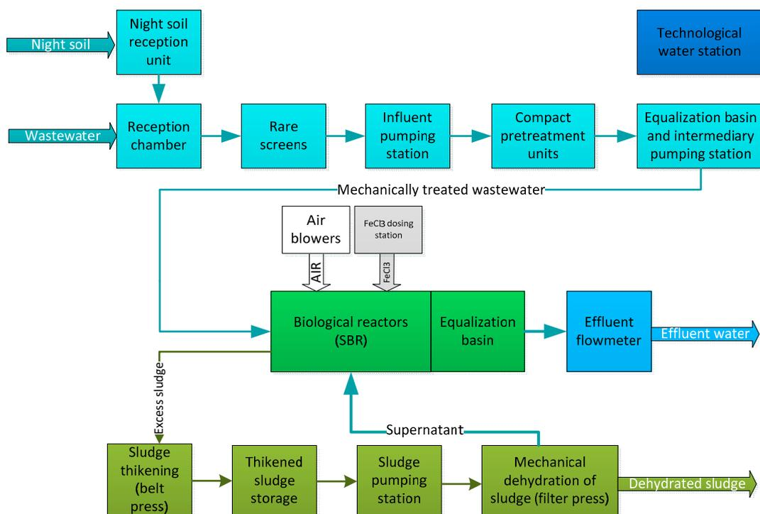
Figure 2. Process flow diagram for WWTP.
