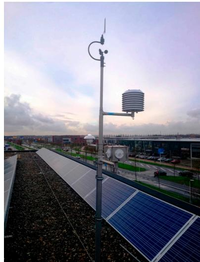
Figure 17. Weather station at the case study building.
