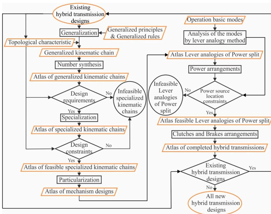
Figure 2. Design procedure for hybrid transmissions.
