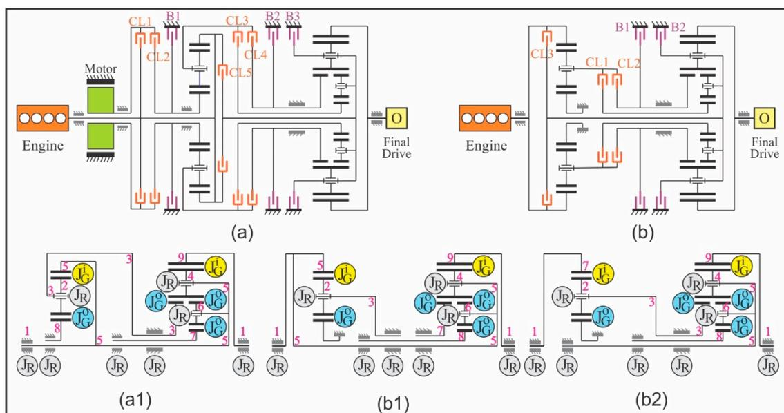
**Figure 3.** Schematic diagrams of existing HT designs: (a) Patent No. US 7,448,975, and (b) ZF-6HP26. Note that (a1) and (b1,b2) show the topological characteristics of (a) and (b), respectively.
