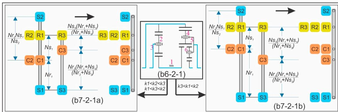
Figure 11. Conversion of transmission mechanisms into compound analogous levers.
