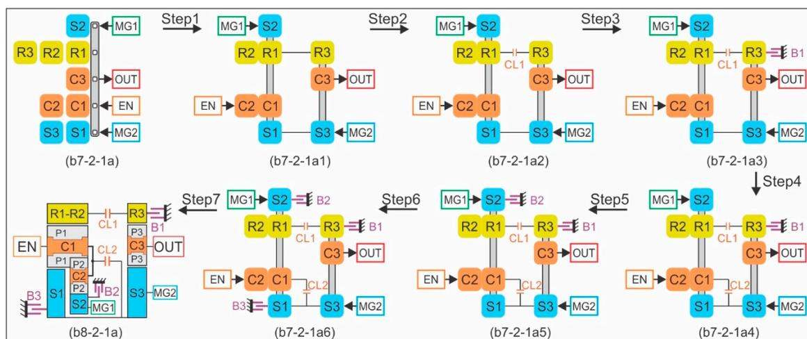
Figure 14. Illustrative example of clutch and brake assignment to feasible levers.
