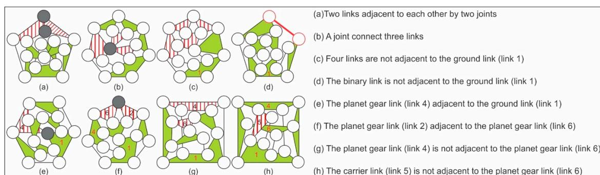
Figure 7. Infeasible generalized kinematic chains.
