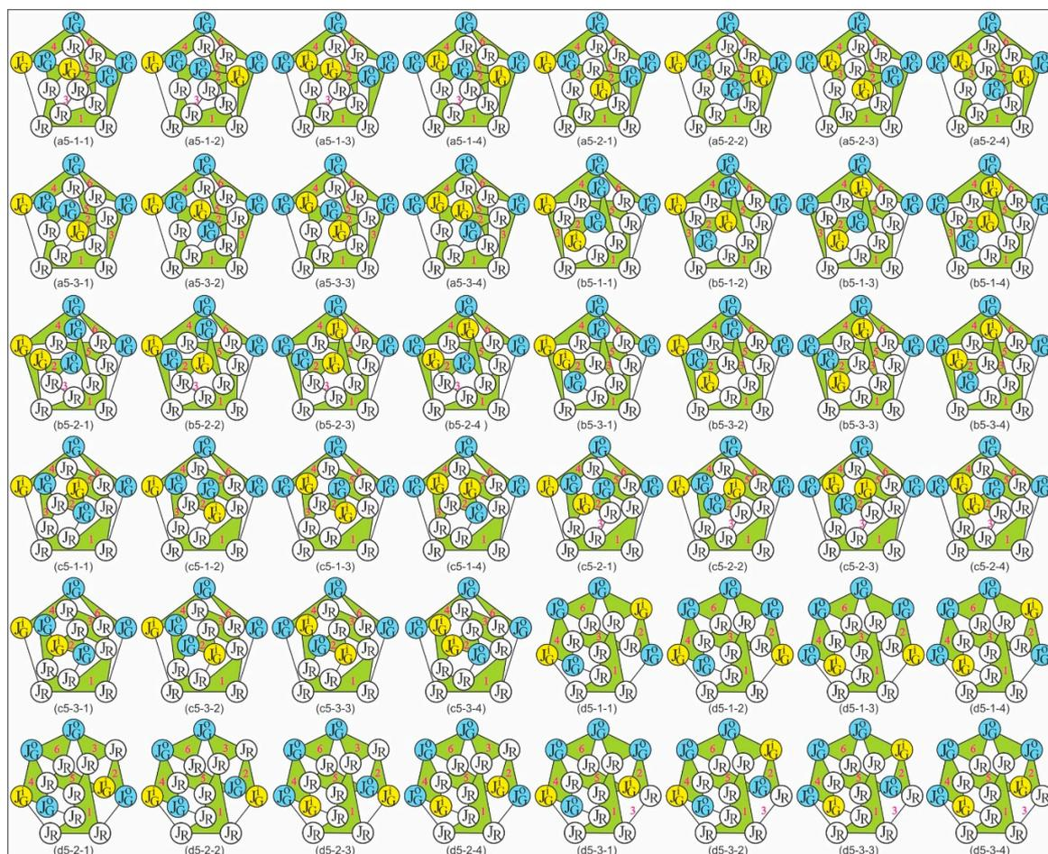
Figure 9. Atlas of feasible specialized kinematic chains.
