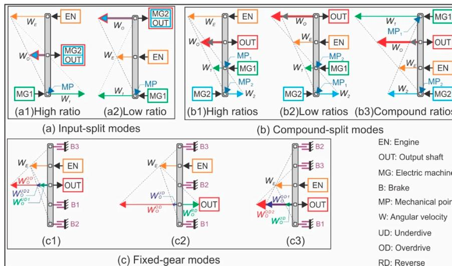
Figure 12. Lever diagrams of different operating modes.
