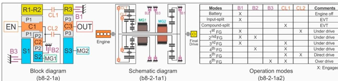
Figure 16. HT system and mode switching diagram considered in kinematic analysis.
