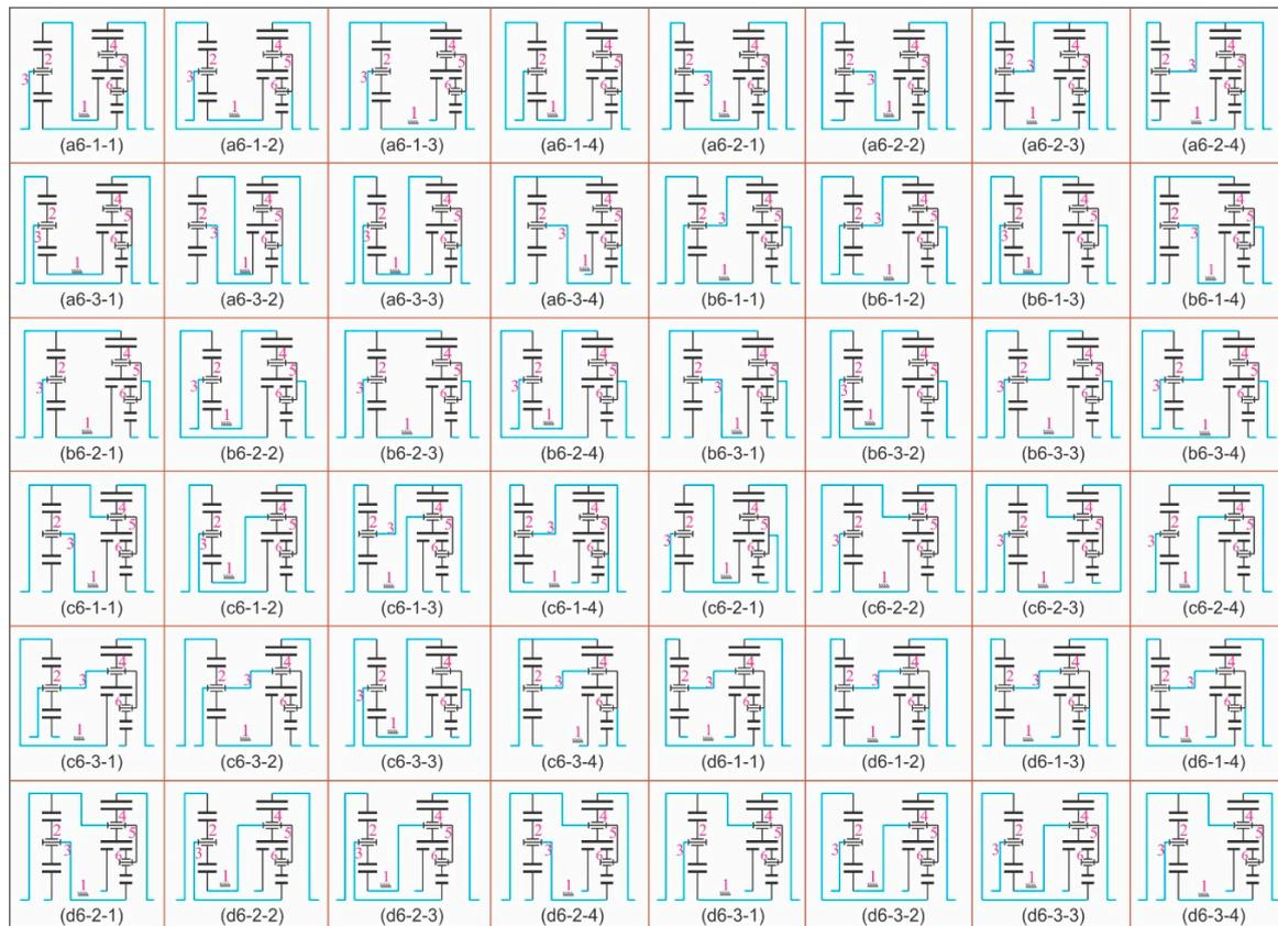
Figure 10. Atlas of transmission mechanism designs.
