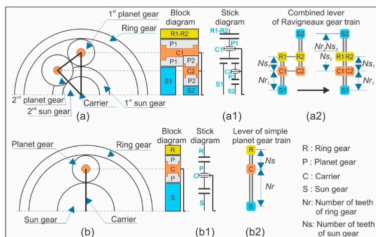
**Figure 1.** Main components of considered HT system: (a) Ravigneaux gear train; (b) simple planetary gear train.
