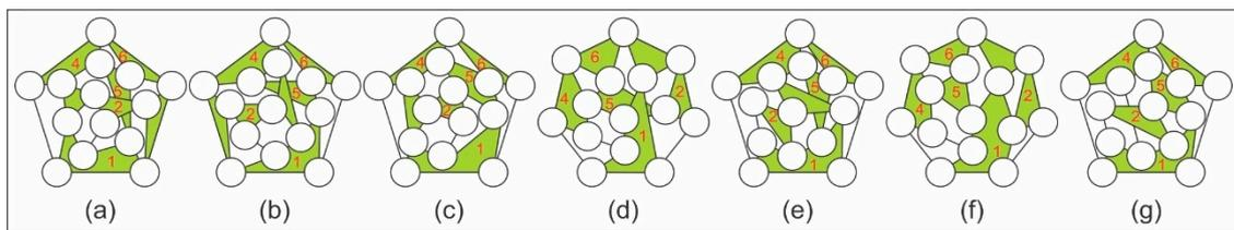
Figure 8. Feasible generalized kinematic chains.
