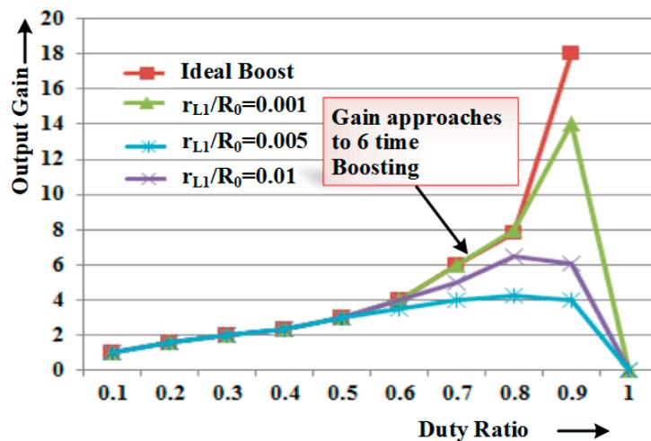
Figure 12. Voltage output gain versus duty cycle.
