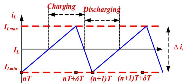
Figure 8. Evolution of the inductor current.
