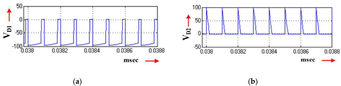
**Figure 17.** Simulation waveforms for input voltage 24V DC and 0.8 duty cycle; (a) voltage across the power diode,  $V_{D1}$  waveform (voltage scale: 50 V/div and t: 20  $\mu$ s/div) and (b) voltage across the power diode,  $V_{D2}$  waveform (voltage scale: 50 V/div and t: 20  $\mu$ s/div).
