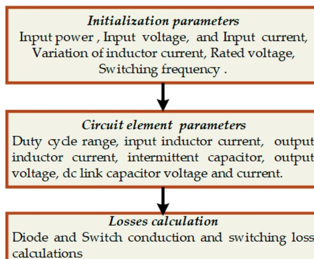
Figure 13. Design setup of converter parameter selections.
