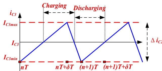
Figure 6. Capacitor current  $i_{C3}$ .
