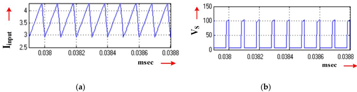
**Figure 15.** Simulation waveforms for input voltage 24V DC and 0.8 duty cycle; (a) input current waveform (current scale: 0.5 A/div and t: 20  $\mu$ s/div) and (b) voltage across the power switch waveform (voltage scale 50 V/div and t: 20  $\mu$ s/div).
