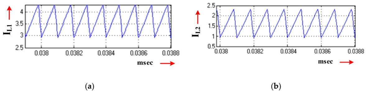
**Figure 16.** Simulation waveforms for input voltage 24 V DC and 0.8 duty cycle; (a) inductor current  $i_{L1}$  waveform (current scale: 0.5 A/div and t: 20  $\mu$ s/div) and (b) inductor current  $i_{L2}$  waveform (current scale: 0.5 A V/div and t: 20  $\mu$ s/div).
