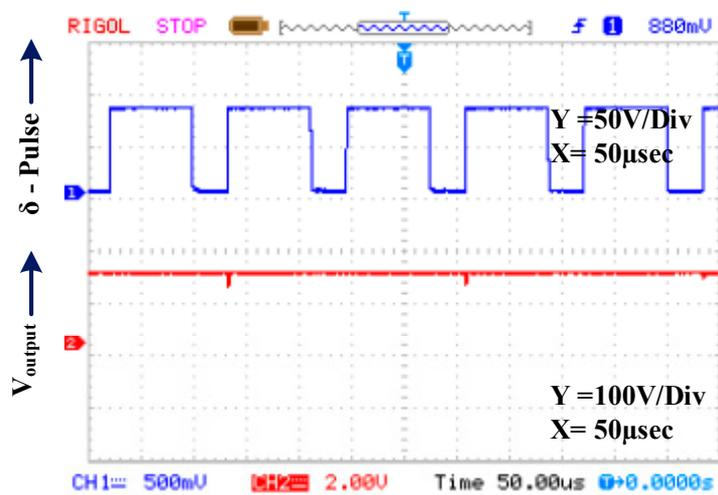
**Figure 20.** The experimental waveform of the duty cycle and input voltage.
