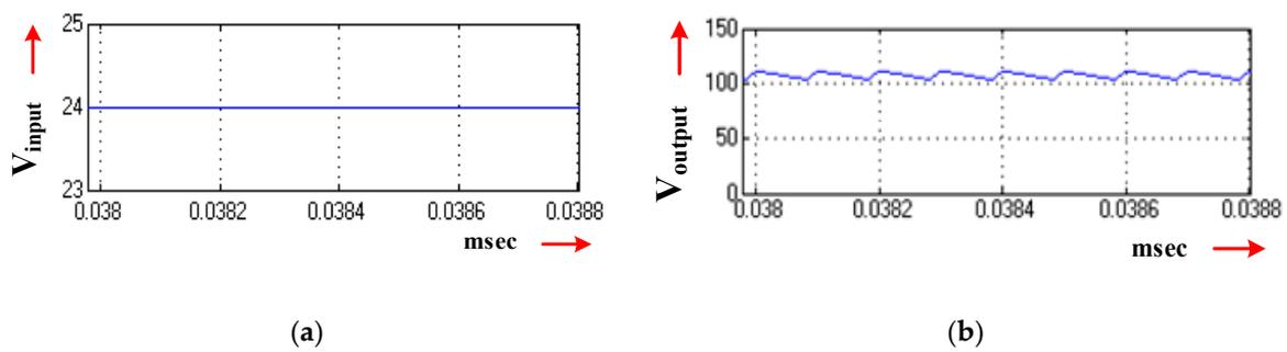
**Figure 14.** Simulation waveforms for input voltage 24V DC and 0.8 duty cycle; (a) input voltage waveform (voltage scale: 1 V/div and t: 20  $\mu$ s/div) and (b) input voltage waveform (voltage scale 50 V/div and t: 20  $\mu$ s/div).
