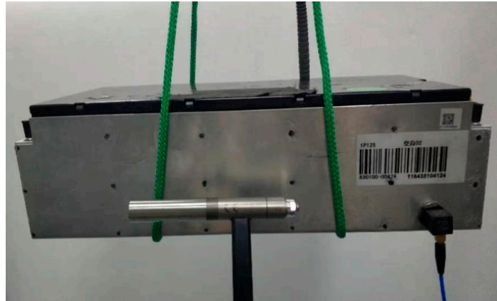
Figure 3. The impulse excitation experiment performed on a battery module.
