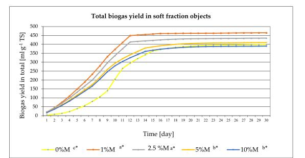
**Figure 1.** Total biogas yield in soft fraction objects. \*Different letters mean statistically significant differences at the significance level p = 0.05.
