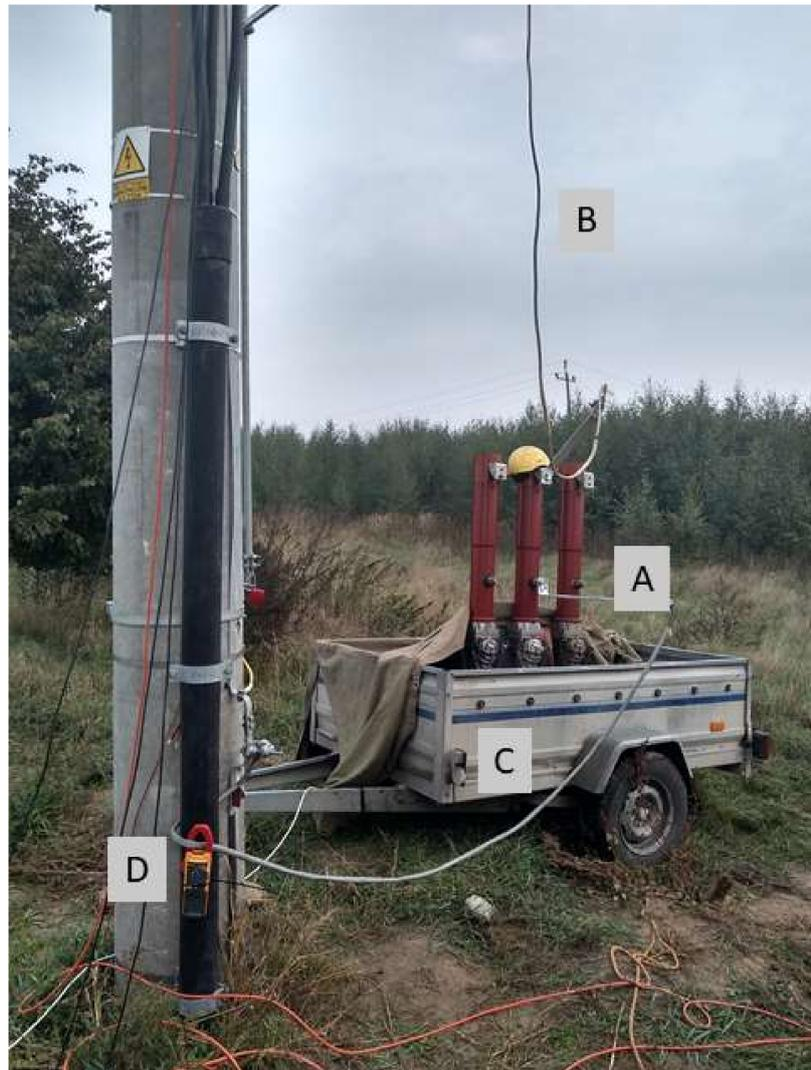
**Figure 3.** Fault test stand: A, remotely controlled circuit breaker; B, connection with MV phase line conductor; C, connection to earthing; and D, measuring system.
