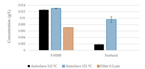
**Figure 1.** Concentration of 5-HMF and furfural in the cellulose pulp hydrolysate after sterilization by three different methods.
