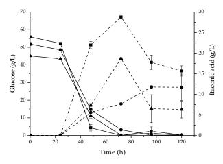
**Figure 2.** Glucose (solid lines) and itaconic acid (dashed lines) concentrations during the fermentation of the cellulose pulp hydrolysate sterilized by different methods. Membrane filter 0.2  $\mu$ m (**I**); autoclave at 112 °C (•); and autoclave at 121 °C (**A**). All the hydrolysates were supplemented with nutrients to be used as fermentation medium.
