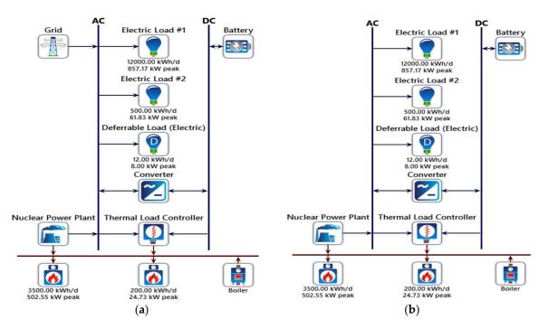
**Figure 11.** (**a**) Small-scale grid-connected stand-alone nuclear energy system; (**b**) Small-scale off-grid stand-alone nuclear energy system.
