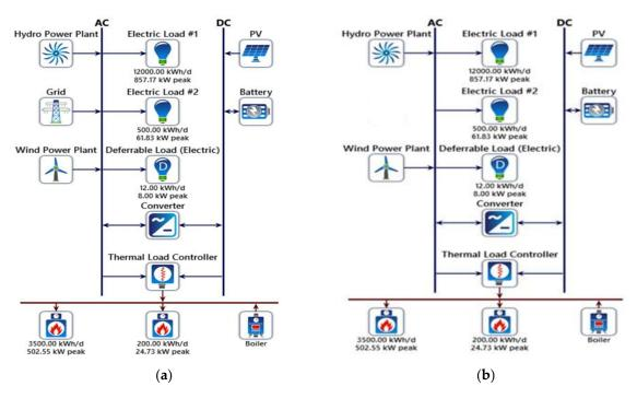
**Figure 9.** (**a**) Small scale stand-alone grid-connected renewable energy sources-based energy system; (**b**) Small scale stand-alone Off-grid renewable energy sources-based energy system.
