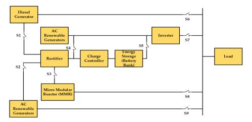
Figure 6. Working strategy of the control algorithm.
