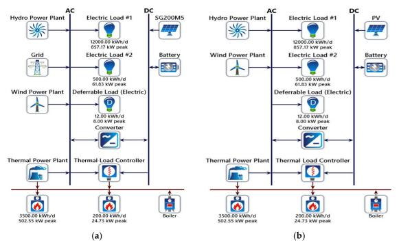
**Figure 10.** (a) Conventional small-scale fossil fuel-based grid-connected thermal and renewable energy sources-based hybrid energy system; (b) Conventional small-scale fossil fuel-based off-grid thermal and renewable energy sources-based hybrid energy system.
