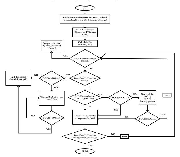
Figure 7. Control algorithm.
