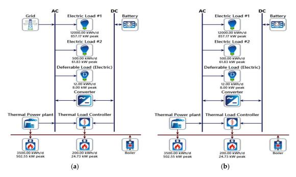
**Figure 8.** (a) Conventional small-scale grid-connected fossil fuel-based thermal energy system; (b) Conventional small-scale Off-grid fossil fuel-based thermal energy system.
