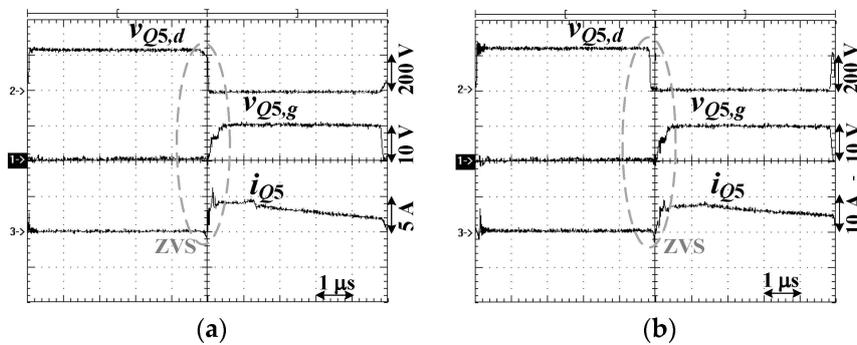
**Figure 12.** Experimental waveforms of  $Q_5$  at (a)  $V_{in} = 240$  V and 50% load and (b)  $V_{in} = 240$  V and 100% load.
