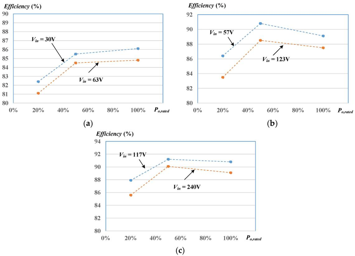
**Figure 13.** Circuit efficiencies under (a) low voltage range ( $V_{in} = 30\text{ V} \sim 63\text{ V}$ ), (b) medium voltage range ( $V_{in} = 57\text{ V} \sim 123\text{ V}$ ), and (c) high voltage range ( $V_{in} = 117\text{ V} \sim 240\text{ V}$ ).
