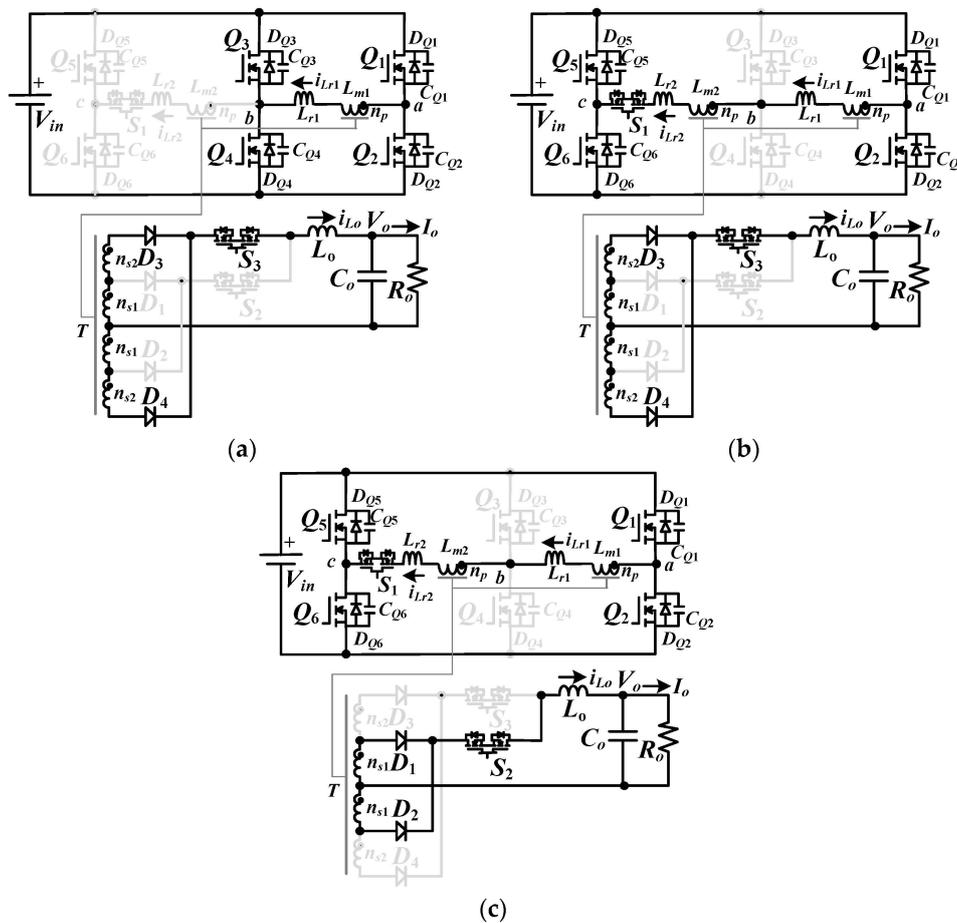
Figure 2. Equivalent circuit of the proposed converter for (a) low voltage range, (b) medium voltage range, and (c) high voltage range.
