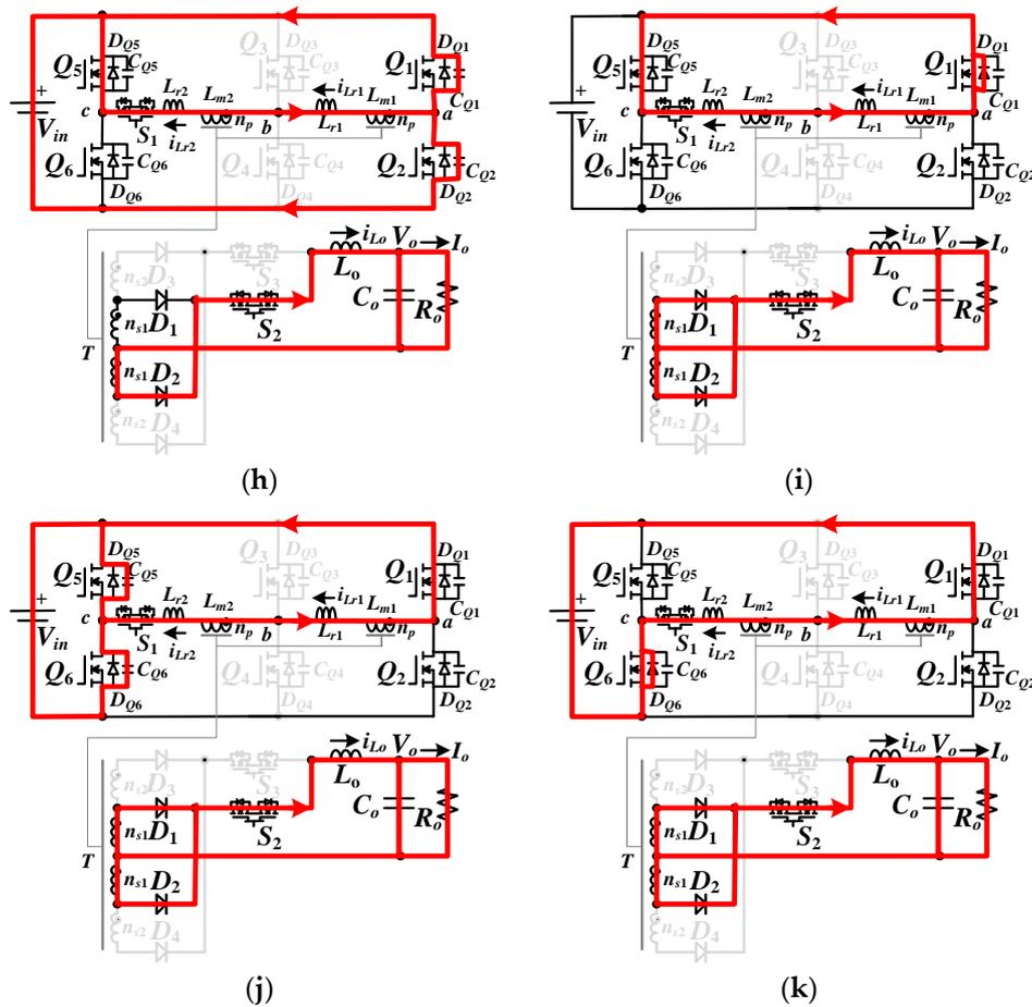
**Figure 5.** PWM waveforms and equivalent circuits at high voltage range operation: (a) PWM voltage and current waveforms for (b) Mode 1, (c) Mode 2, (d) Mode 3, (e) Mode 4, (f) Mode 5, (g) Mode 6, (h) Mode 7, (i) Mode 8, (j) Mode 9, and (k) Mode 10.
