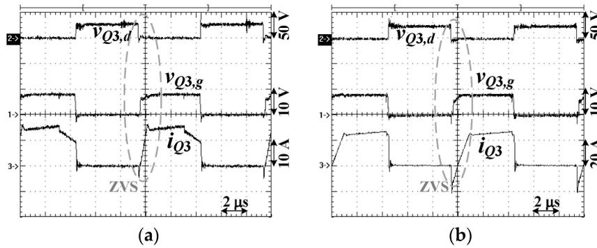
**Figure 11.** Experimental waveforms of  $Q_3$  at (a)  $V_{in} = 30$  V and 50% load and (b)  $V_{in} = 30$  V and 100% load.
