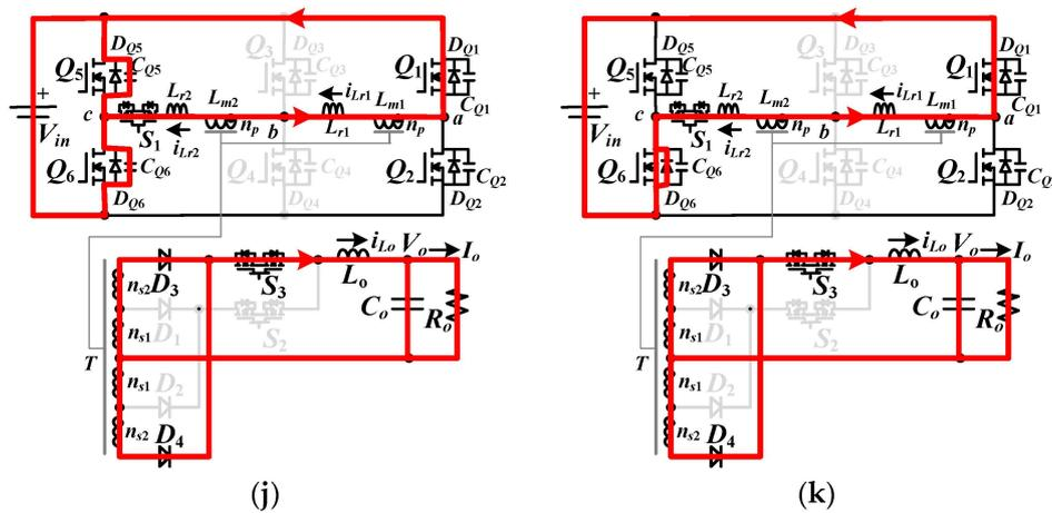
**Figure 4.** PWM waveforms and equivalent circuits at medium voltage range operation: (a) PWM voltage and current waveforms for (b) Mode 1, (c) Mode 2, (d) Mode 3, (e) Mode 4, (f) Mode 5, (g) Mode 6, (h) Mode 7, (i) Mode 8, (j) Mode 9, and (k) Mode 10.
