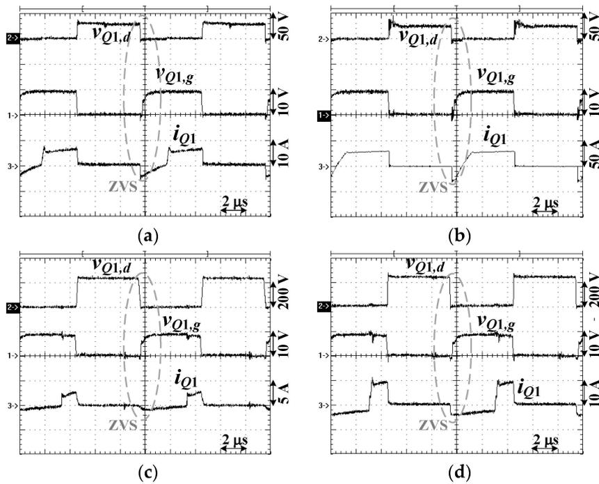
**Figure 10.** Experimental waveforms of  $Q_1$  at (a)  $V_{in} = 30$  V and 20% load, (b)  $V_{in} = 30$  V and 100% load, (c)  $V_{in} = 240$  V and 20% load, and (d)  $V_{in} = 240$  V and 100% load.
