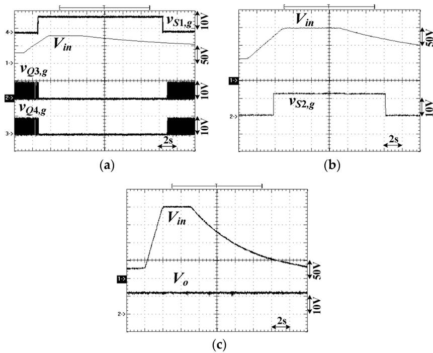
**Figure 14.** Measured waveforms under full load (a)  $V_{in}$ ,  $v_{S1,g}$ ,  $v_{Q3,g}$ ,  $v_{Q4,g}$ , (b)  $V_{in}$ ,  $v_{S2,g}$ , and (c)  $V_{in}$ ,  $V_o$ .
