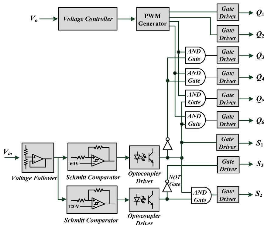
Figure 6. Control block of the studied converter.
