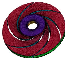
(a) Mesh of the impeller.
