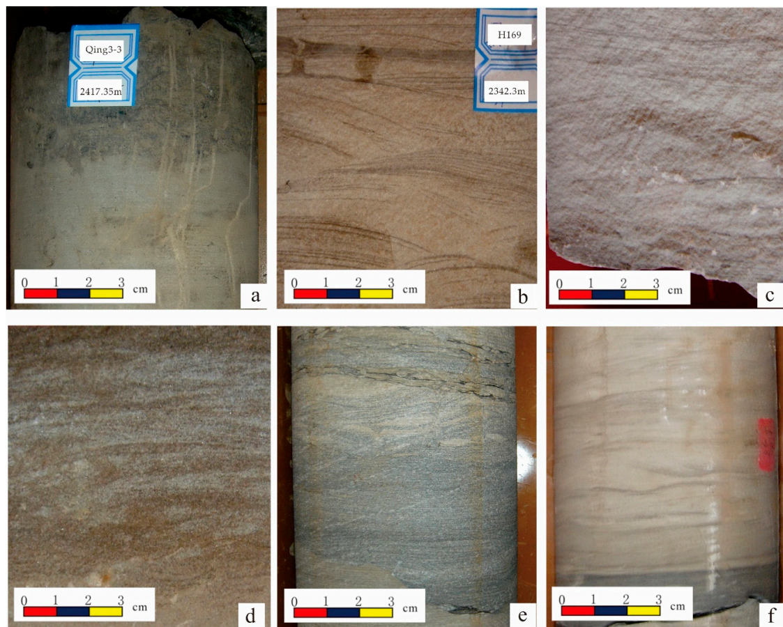
Figure 4. Photographs of cores of storm sediments. (a) Qing3-3, 2417.35m, scouring filling structure; (b) H169, 2341.3m, hummocky cross bedding; (c) H169, 2350.1m, hummocky cross bedding; (d) H169, 2342.5m, hummocky cross bedding; (e) H84, 2457.8m, slot mold structure; (f) H102, 2419.1m, wave ripple cross bedding.
