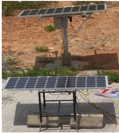
Figure 1. Sun tracking and fixed-tilted PV systems.
