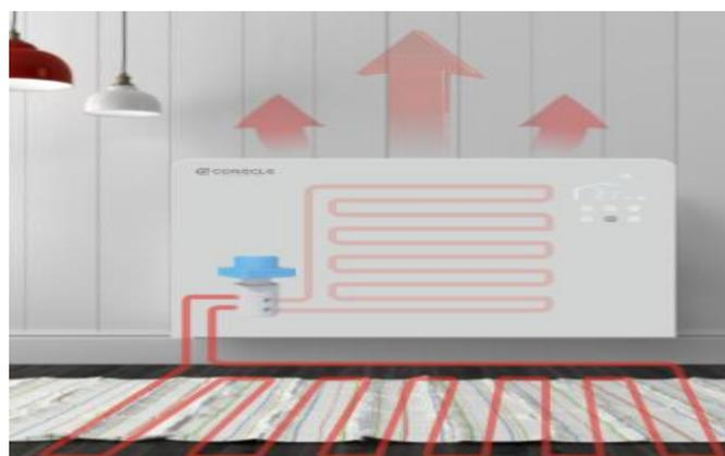
Figure 1. Floor radiation-convection combined heating system.
