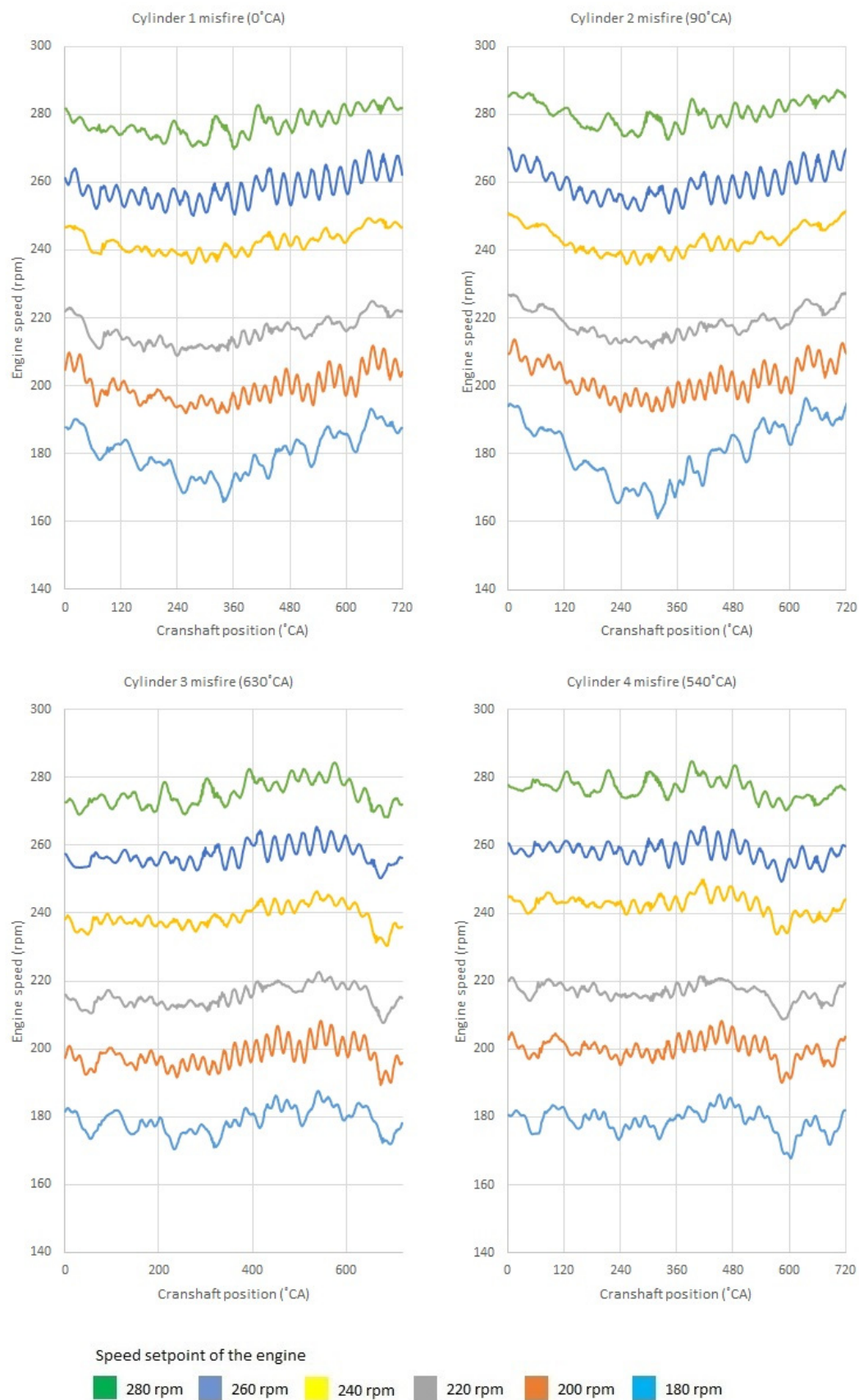
Figure 13. Instantaneous speed ranges at the time of combustion loss in cylinders 1–4 of a Buckau-Wolf R8DV-136 engine with pre-set speeds of 180–280 rpm.
