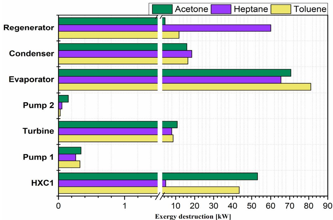
**Figure 3.** Fraction of exergy destroyed per component.
