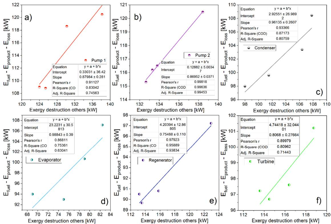
**Figure 4.** Endogenous destruction of exergy of acetone (a) Pump 1, (b) Pump 2, (c) condenser, (d) evaporator, (e) regenerator, and (f) turbine.
