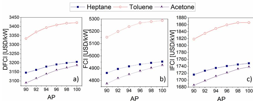
**Figure 8.** Effect of evaporator pinch point on investment costs for a RORC system varying (a) DFCI, (b) FCI, and (c) IFCI.
