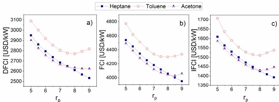
**Figure 6.** Effect of pressure ratio on investment costs for a RORC system varying (a) DFCI, (b) FCI, and (c) IFCI.
