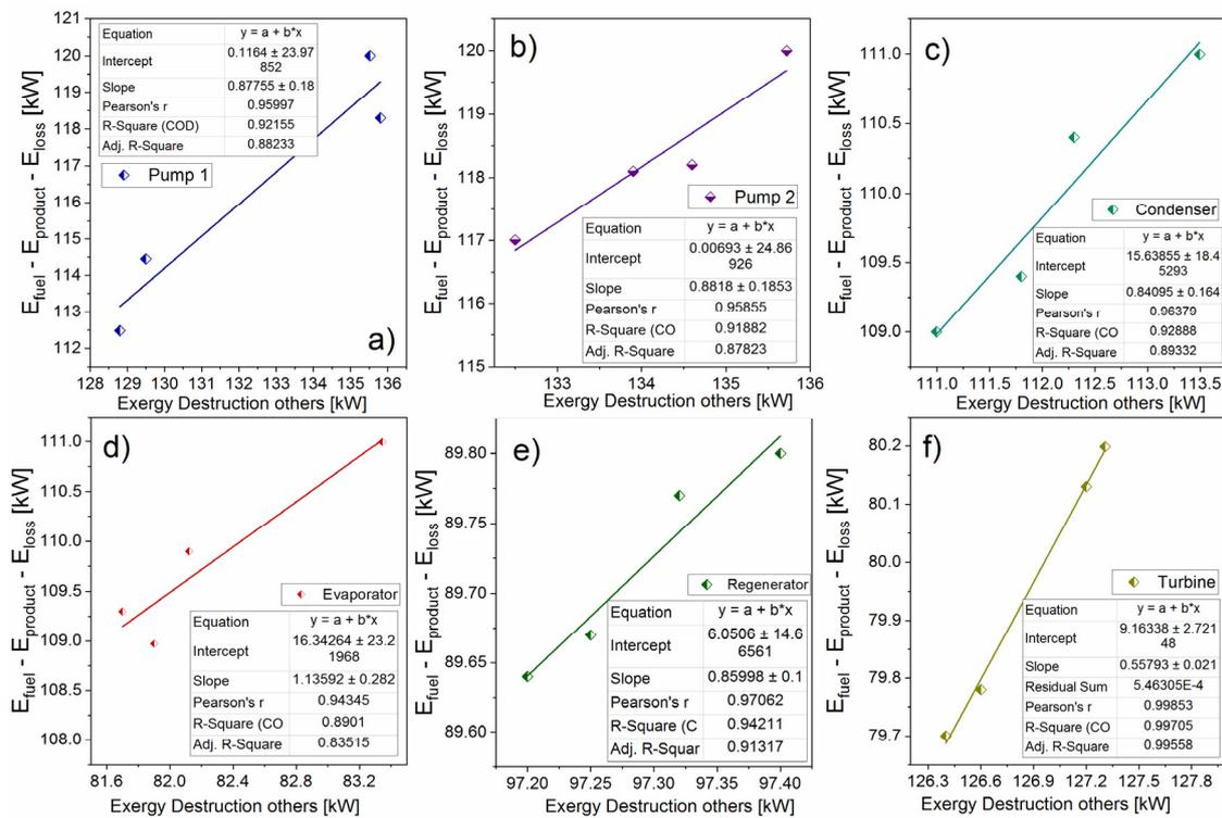
**Figure A1.** Endogenous destruction of exergy for heptane (a) Pump 1, (b) Pump 2, (c) condenser, (d) evaporator, (e) regenerator, and (f) turbine.
