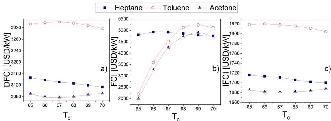
**Figure 7.** Effect of condensing temperature on investment costs for a RORC system varying (a) DFCI, (b) FCI, and (c) IFCI.
