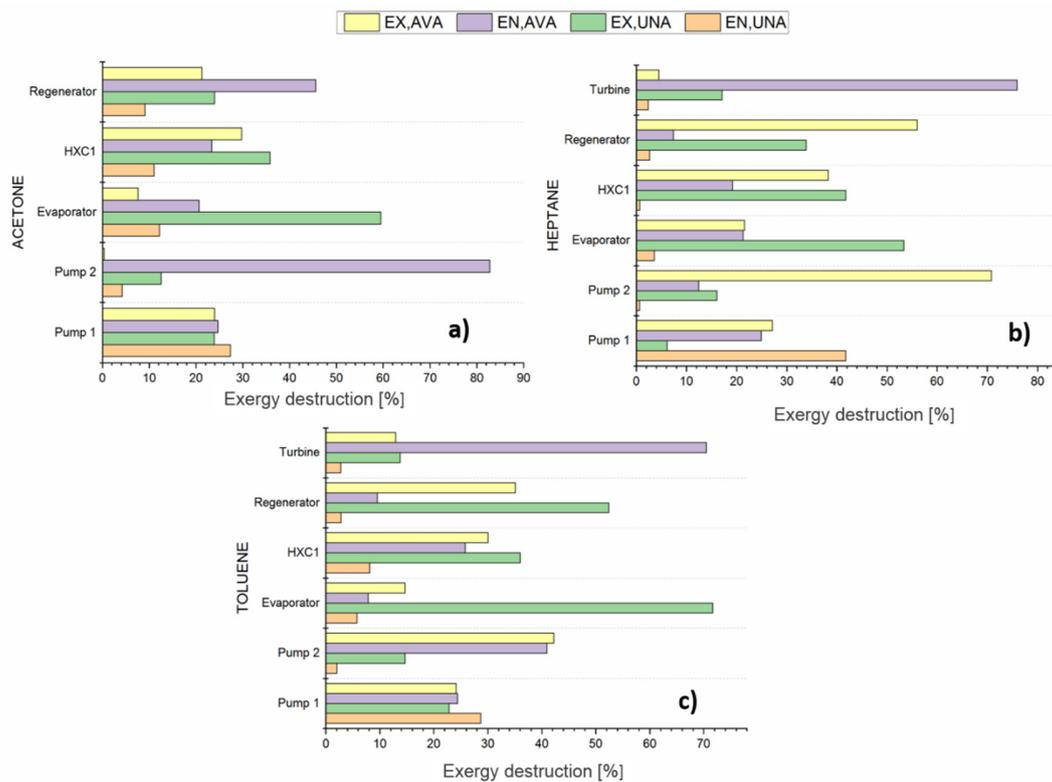
**Figure 5.** Disaggregation of exergy into the avoidable and unavoidable endogenous part and avoidable and unavoidable exogenous part for (a) acetone, (b) heptane, and (c) toluene.
