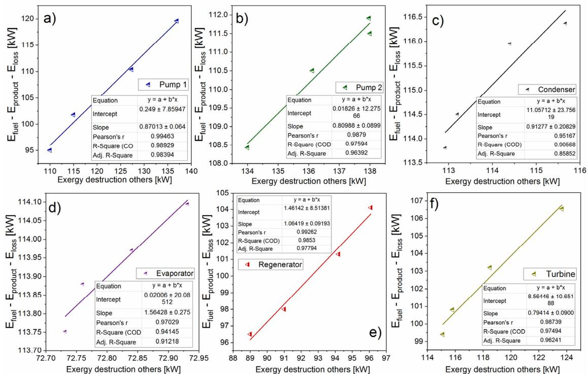
**Figure A2.** Endogenous destruction of exergy for toluene (a) Pump 1, (b) Pump 2, (c) condenser, (d) evaporator, (e) regenerator, and (f) turbine.
