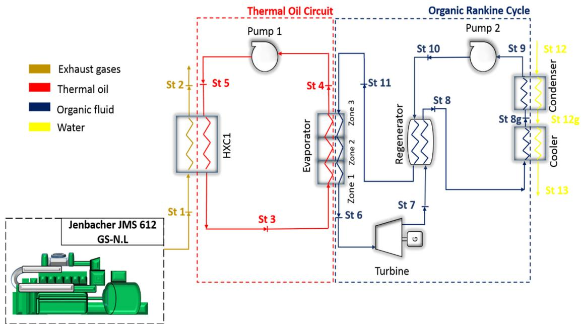
**Figure 1.** Schematic diagram of the Jenbacher JMS engine integration to the thermal oil cycle configuration and organic Rankine cycle.
