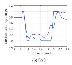
**Figure 21.** Mechanical torque of DGs of microgrid C (island mode) in: storage (**a**) and sun and storage (**b**) scenario.
