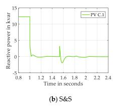
**Figure 26.** Reactive power of PV of microgrid C (island mode) in: storage (a) and sun and storage (b) scenario.
