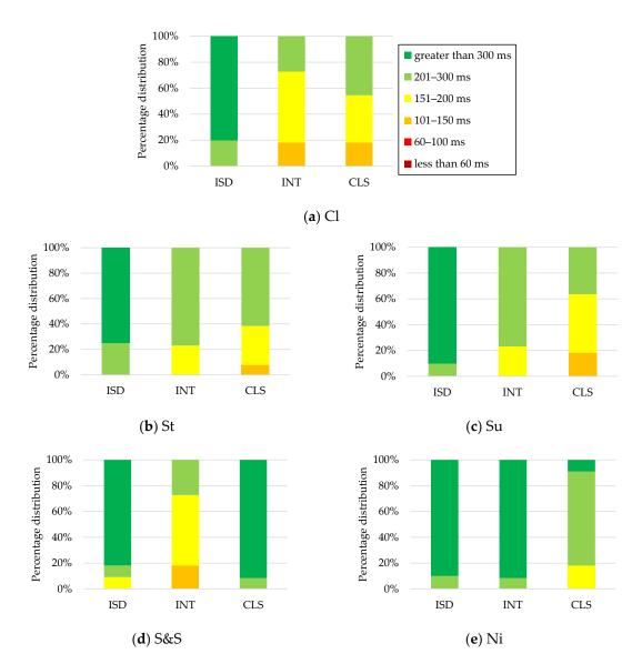
**Figure 14.** Percentage distribution of *CCT* in microgrid C with respect to different operating modes in: classical (**a**), storage (**b**), sun (**c**), sun and storage (**d**), and night (**e**) scenario.
