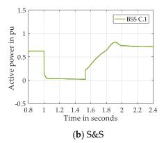
**Figure 24.** Real power of BSS of microgrid C (island mode) in: storage (**a**) and sun and storage (**b**) scenario.
