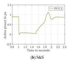
**Figure 23.** Real power of PV of microgrid C (island mode) in: storage (a) and sun and storage (b) scenario.
