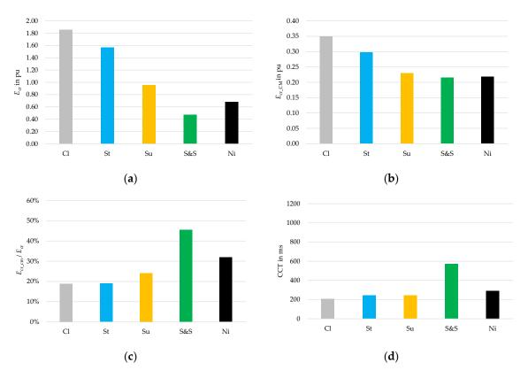
**Figure 37.** Analysis of the critical energies in the clustered mode: system critical energy ( $\mathbf{a}$ ), critical energy of the critical machine ( $\mathbf{b}$ ), ratio of the critical energies ( $\mathbf{c}$ ), and *CCT* ( $\mathbf{d}$ ).
