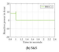
**Figure 27.** Reactive power of BSS of microgrid C (island mode) in: storage (**a**) and sun and storage (**b**) scenario.
