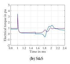
**Figure 20.** Electrical torque of DGs of microgrid C (island mode) in: storage (**a**) and sun and storage (**b**) scenario.
