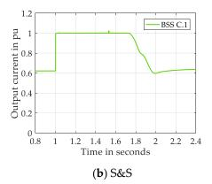
**Figure 30.** Current of BSS of microgrid C (island mode) in: storage (a) and sun and storage (b) scenario.
