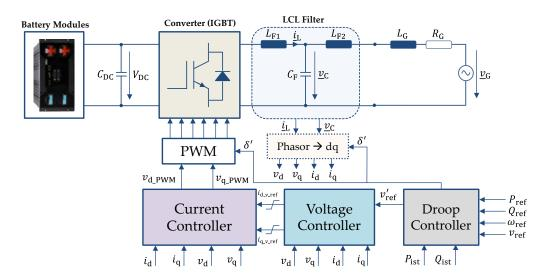
Figure 7. Block diagram of grid-forming BSS with corresponding controllers, according to [36,42].
