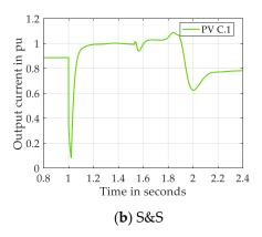
Figure 29. Current of PV of microgrid C (island mode) in: storage (a) and sun and storage (b) scenario.
