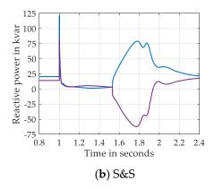
**Figure 25.** Reactive power of DGs of microgrid C (island mode) in: storage (a) and sun and storage (b) scenario.
