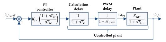
Figure 4. Block diagram of the inner control loop in PV, according to [35].
