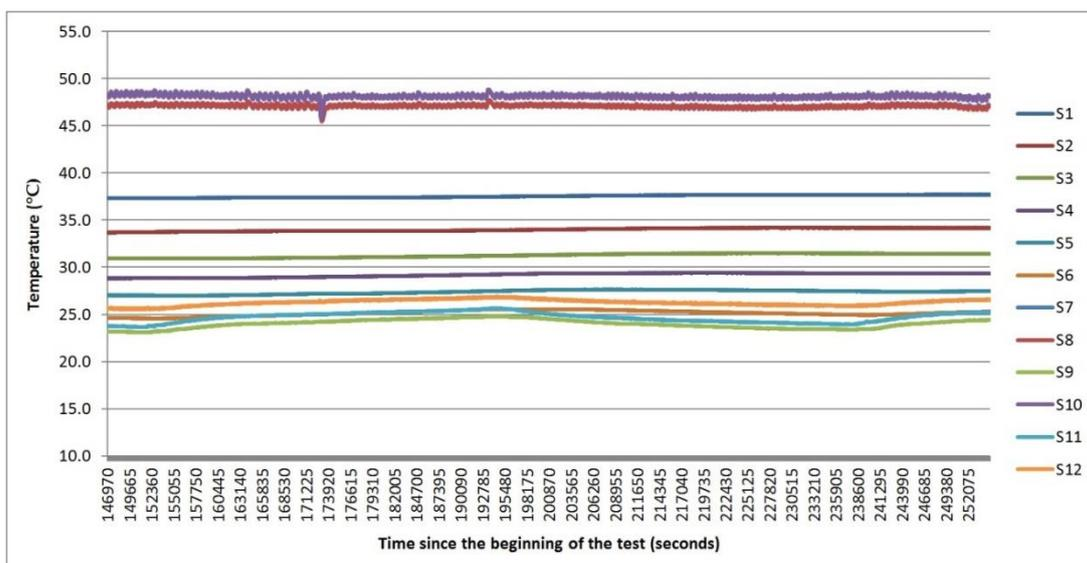
**Figure 10.** Corrected temperature measurements in the permanent regime by applying the correction factors on sensors S1–S10. (Note that S7 measurements are hidden due to their coincidence with the measurements from S8).
