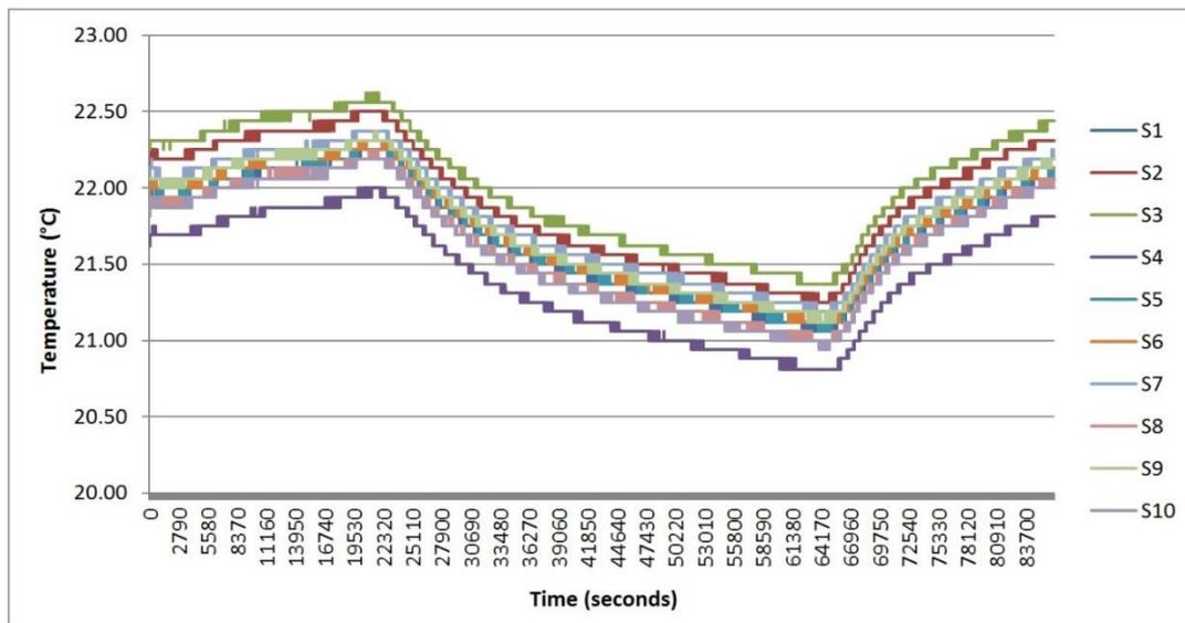
Figure 6. Temperature sensors measuring in a common ambient for the corresponding calibration.
