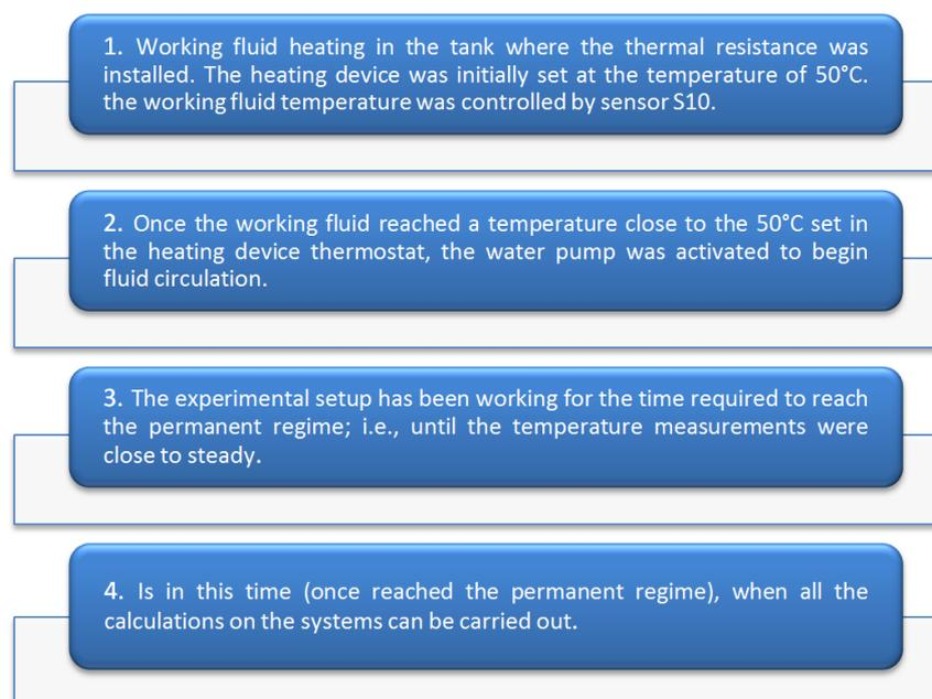
**Figure 7.** Description of the experimental methodology followed on the geothermal device.
