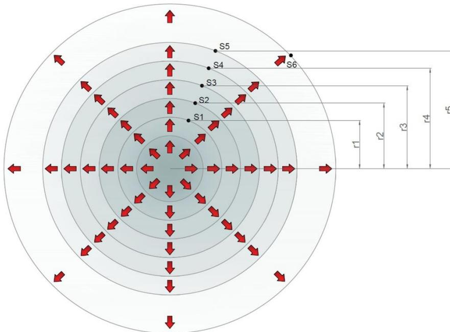
**Figure 4.** Heat transmission through the ground system and temperature sensors location.
