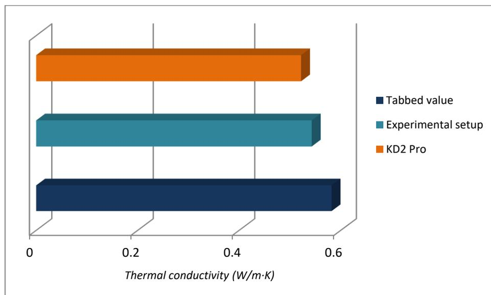
**Figure 14.** Thermal conductivity of the sandy material obtained from the experimental setup, the KD2 Pro device, and the standard tabulated value.
