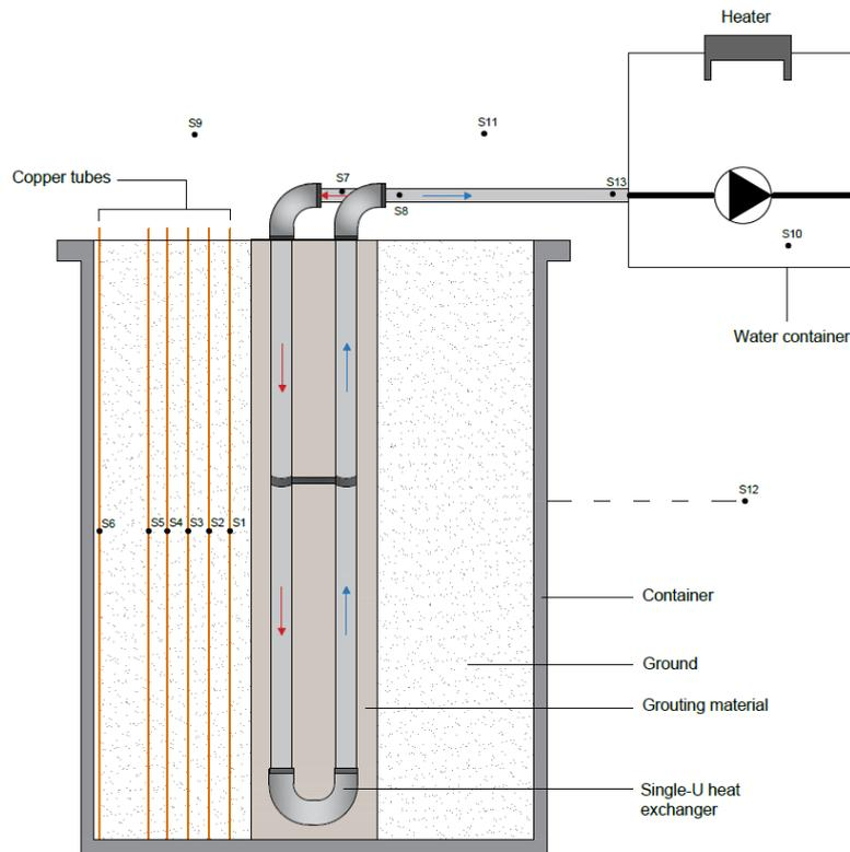
Figure 1. Schema of the geothermal setup reproduced in the laboratory.
