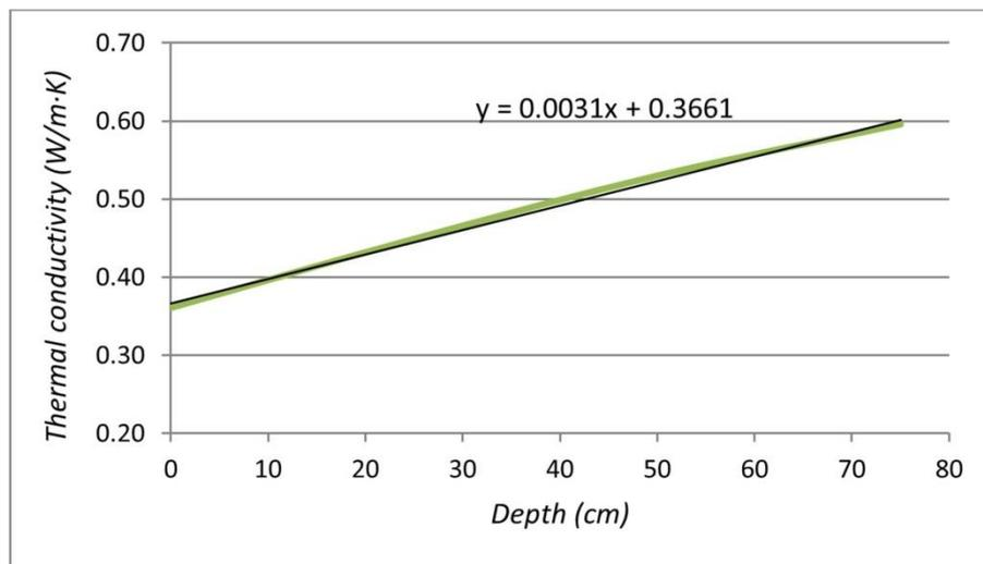
**Figure 13.** Relation between the thermal conductivity of the material and the depth where the parameter was measured.
