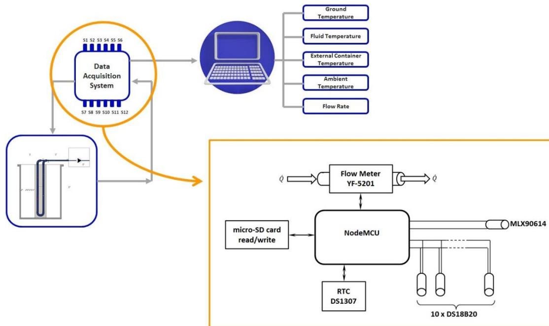
**Figure 3.** Schema of the data acquisition system.
