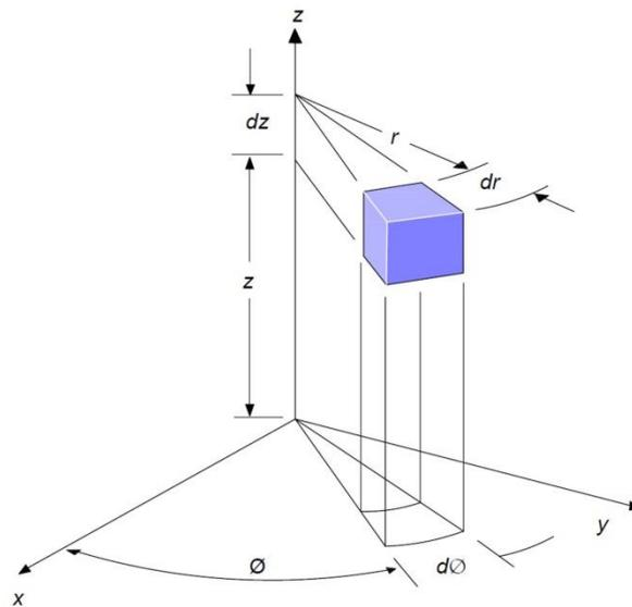
Figure 5. A differential volume element in cylindrical coordinates [30].
