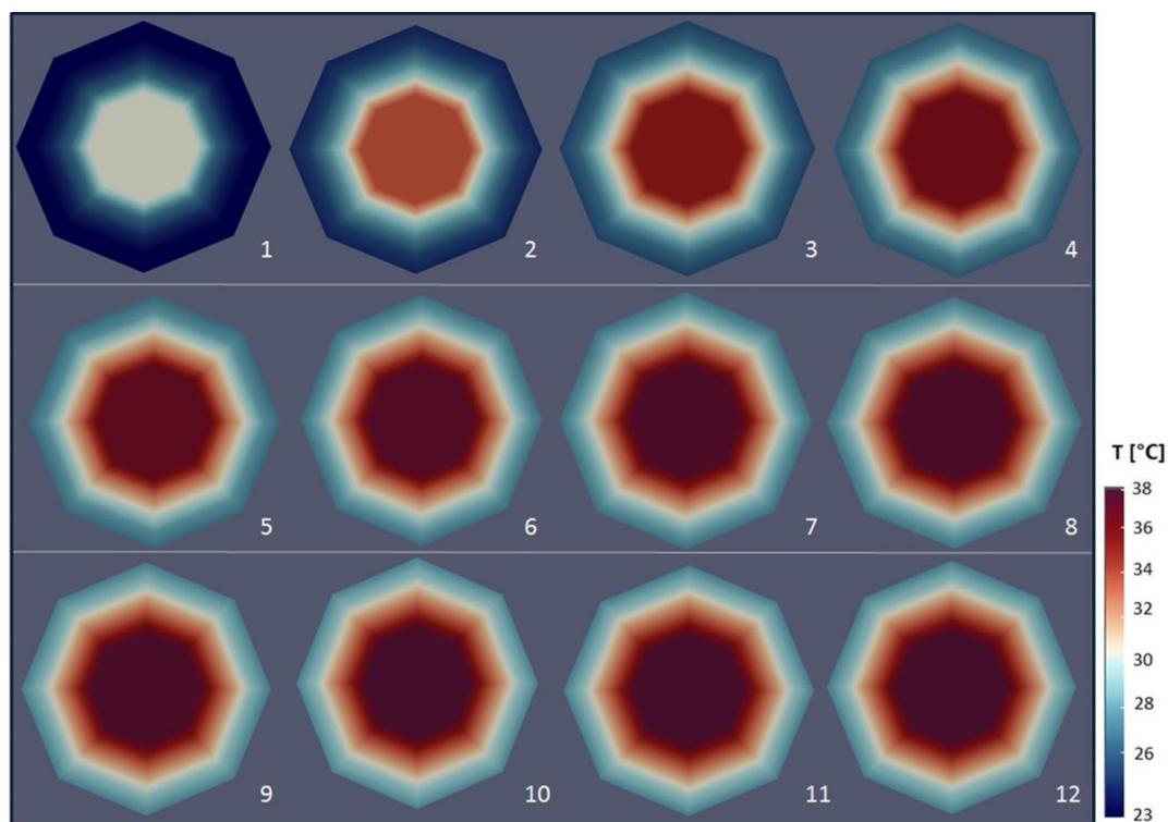
**Figure 11.** Heat transfer between the working fluid (water) and the surrounding material (silica sand with 15% humidity) according to the temperature values recorded by sensors S1–S5: Step 1 = 21,600 s, step 2 = 43,200 s, step 3 = 64,800 s, step 4 = 86,400 s, step 5 = 108,000 s, step 6 = 129,600 s, step 7 = 151,200 s, step 8 = 172,800 s, step 9 = 194,400 s, step 10 = 216,000 s, step 11 = 237,600, and step 12 = 259,200.
