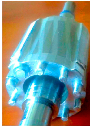
Figure 5. The manufactured rotor with milled slots.
