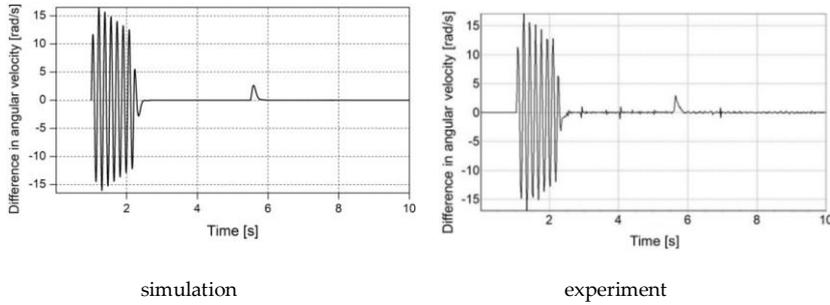
Figure 10. Difference in angular velocity vs. time.
