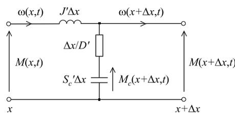
Figure 3. Equivalent circuit of a transmission shaft section.
