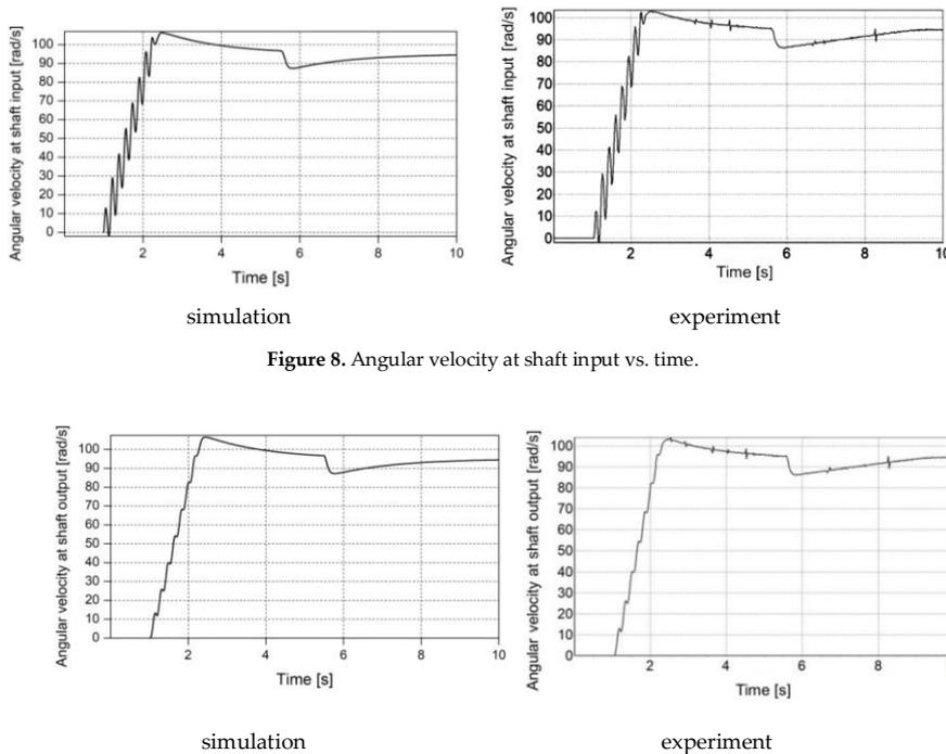
**Figure 8.** Angular velocity at shaft input vs. time.
