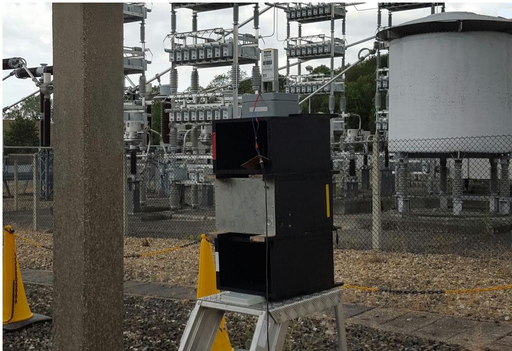
Figure 6. Experimental setup showing the arrangement adopted for the FM directly underneath the busbar connected to the charged cable.
