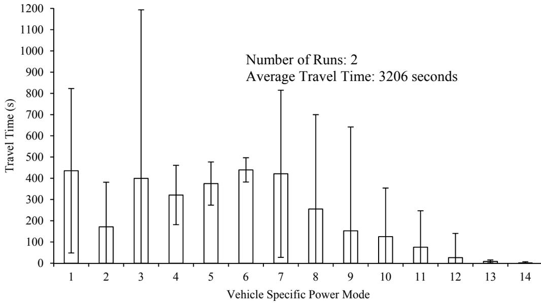
Figure S8 The Travel Time Distribution in Each Vehicle Specific Power Mode for Route 2
