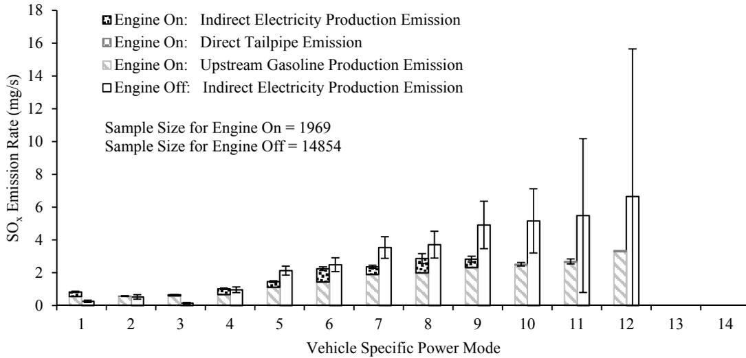
Figure S33 The Oxide of Sulfur (SO<sub>x</sub>) Emission Rate Versus Vehicle Specific Power (VSP) Mode for Engine On and Off for Charge Depleting (CD) Mode for a 2013 Toyota Prius Plug-In Hybrid Measured from January 18, 2013 to January 25, 2013 in Raleigh/Research Triangle Park, North Carolina Area
