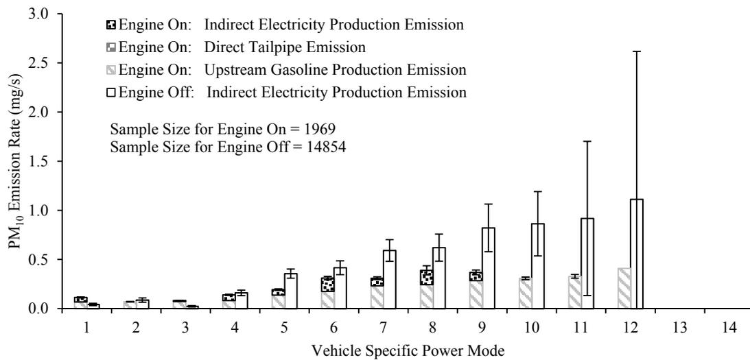
Figure S35 The Particulate Matter with Diameters of 10 Micrometers or Less (PM<sub>10</sub>) Emission Rate Versus Vehicle Specific Power (VSP) Mode for Engine On and Off for Charge Depleting (CD) Mode for a 2013 Toyota Prius Plug-In Hybrid Measured from January 18, 2013 to January 25, 2013 in Raleigh/Research Triangle Park, North Carolina Area
