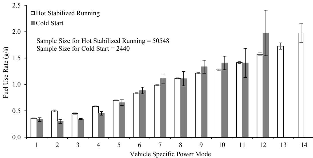
Figure S50 The Average Fuel Use Rate Versus Vehicle Specific Power (VSP) Mode for Cold Start and Hot Stabilized Running During Engine On for a 2013 Toyota Prius Plug-In Hybrid Measured from January 18, 2013 to January 25, 2013 in Raleigh/Research Triangle Park, North Carolina Area
