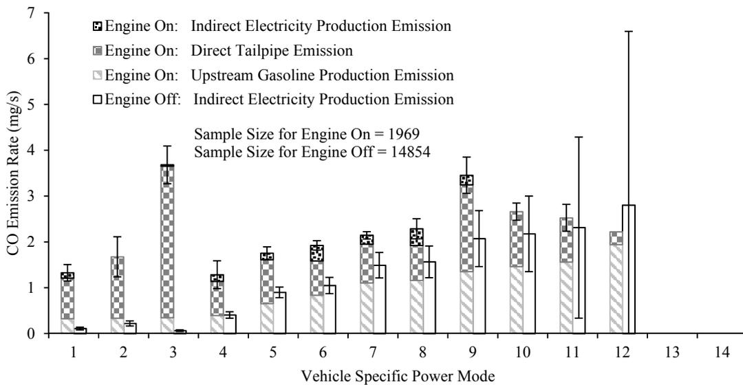
Figure S30 The Carbon Monoxide (CO) Emission Rate Versus Vehicle Specific Power (VSP) Mode for Engine On and Off for Charge Depleting (CD) Mode for a 2013 Toyota Prius Plug-In Hybrid Measured from January 18, 2013 to January 25, 2013 in Raleigh/Research Triangle Park, North Carolina Area
