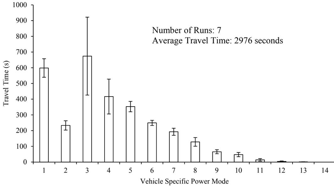
Figure S2 The Travel Time Distribution in Each Vehicle Specific Power Mode for Route A
