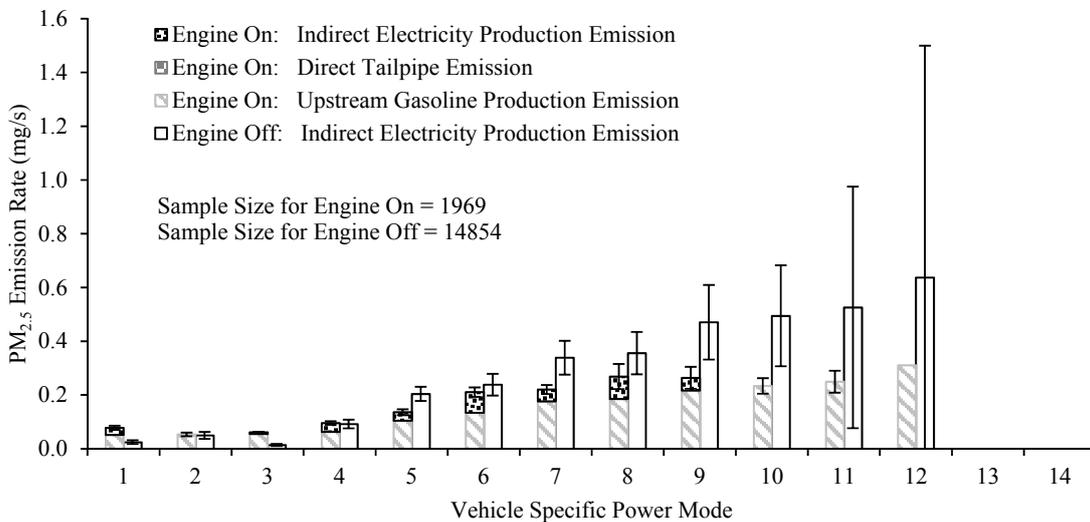
Figure S34 The Particulate Matter with Diameters of 2.5 Micrometers or Less (PM<sub>2.5</sub>) Emission Rate Versus Vehicle Specific Power (VSP) Mode for Engine On and Off for Charge Depleting (CD) Mode for a 2013 Toyota Prius Plug-In Hybrid Measured from January 18, 2013 to January 25, 2013 in Raleigh/Research Triangle Park, North Carolina Area
