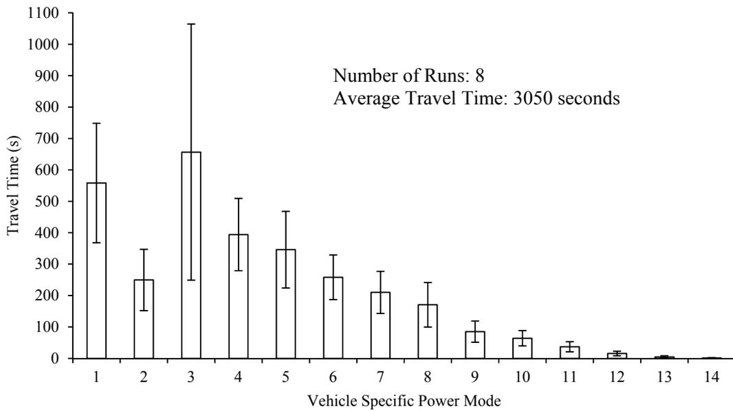
Figure S4 The Travel Time Distribution in Each Vehicle Specific Power Mode for Route C
