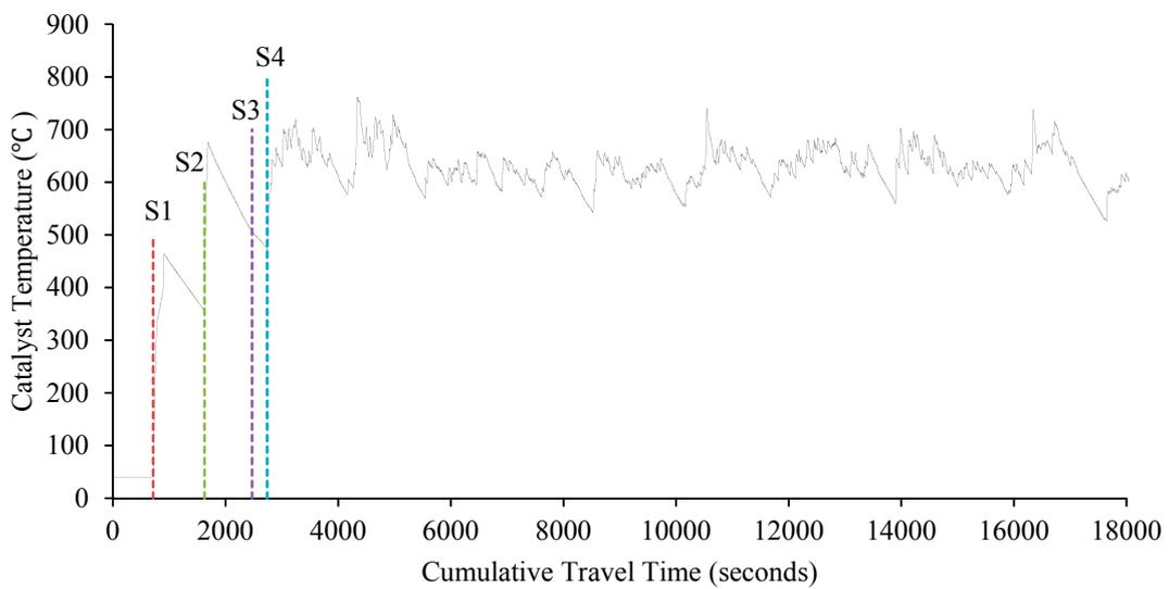
Figure S45 Second-by-Second the Catalyst Temperature Data for a 2013 Toyota Prius Plug-In Hybrid Measured on January 21, 2013 in Raleigh/Research Triangle Park, NC Area
