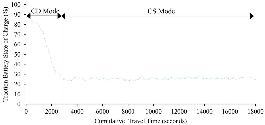
Figure S10 Second-by-Second the Traction Battery State of Charge Data for Charge Depleting (CD) and Charge Sustaining (CS) Modes for a 2013 Toyota Prius Plug-In Hybrid Measured on January 21, 2013 in Raleigh/Research Triangle Park, NC Area
