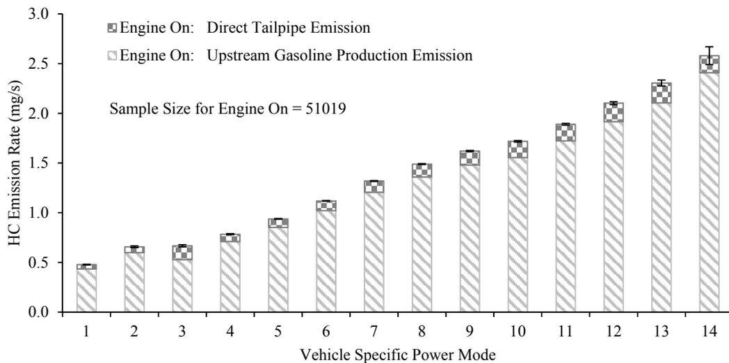
Figure S39 The Hydrocarbon (HC) Emission Rate Versus Vehicle Specific Power (VSP) Mode for Engine On for Charge Sustaining (CS) Mode for a 2013 Toyota Prius Plug-In Hybrid Measured from January 18, 2013 to January 25, 2013 in Raleigh/Research Triangle Park, North Carolina Area
