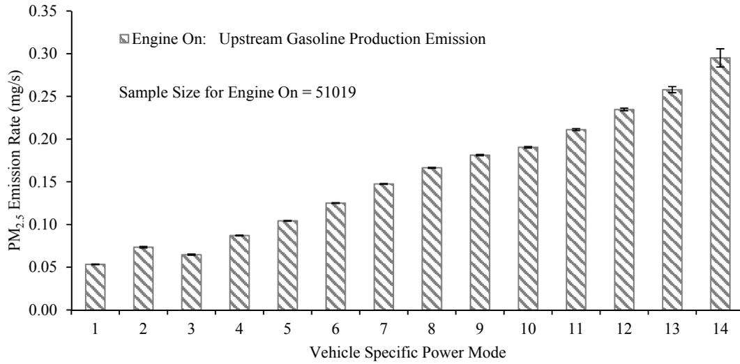
Figure S42 The Particulate Matter with Diameters of 2.5 Micrometers or Less (PM<sub>2.5</sub>) Emission Rate Versus Vehicle Specific Power (VSP) Mode for Engine On for Charge Sustaining (CS) Mode for a 2013 Toyota Prius Plug-In Hybrid Measured from January 18, 2013 to January 25, 2013 in Raleigh/Research Triangle Park, North Carolina Area
