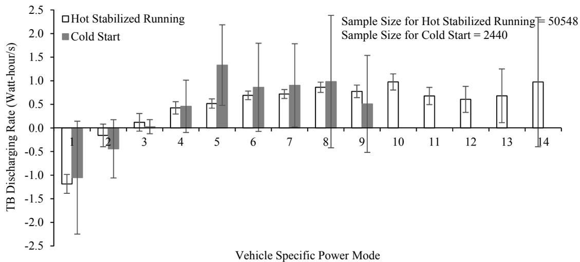
Figure S49 The Average Traction Battery (TB) Discharging Rate Versus Vehicle Specific Power (VSP) Mode for Cold Start and Hot Stabilized Running During Engine On for a 2013 Toyota Prius Plug-In Hybrid Measured from January 18, 2013 to January 25, 2013 in Raleigh/Research Triangle Park, North Carolina Area
