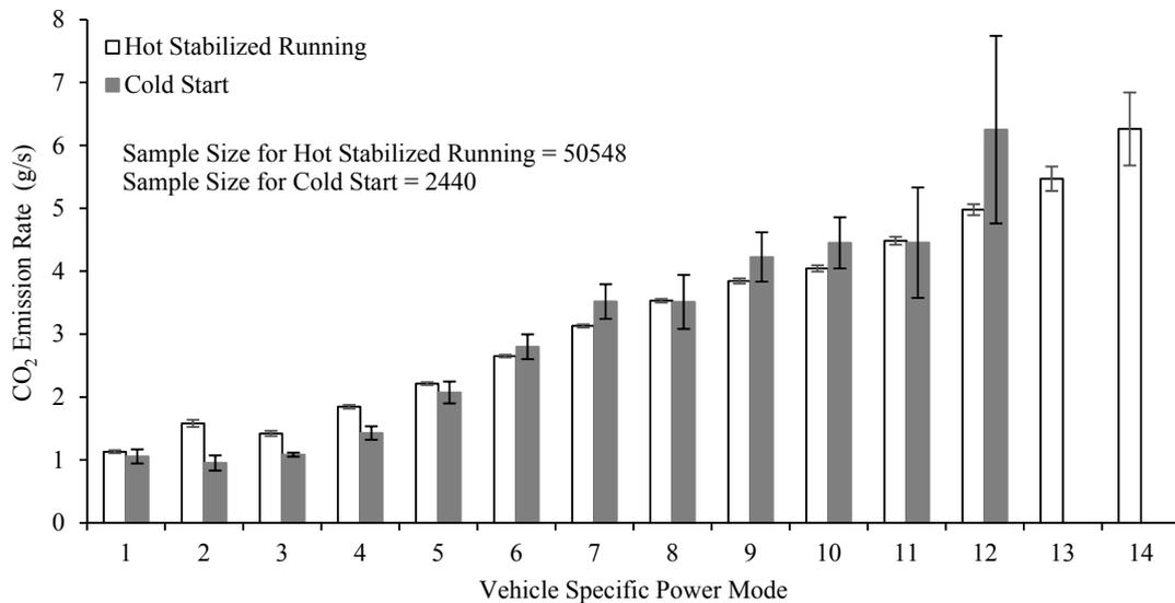
Figure S51 The Average Tailpipe Carbon Dioxide (CO<sub>2</sub>) Emission Rate Versus Vehicle Specific Power (VSP) Mode for Cold Start and Hot Stabilized Running During Engine On for a 2013 Toyota Prius Plug-In Hybrid Measured from January 18, 2013 to January 25, 2013 in Raleigh/Research Triangle Park, North Carolina Area
