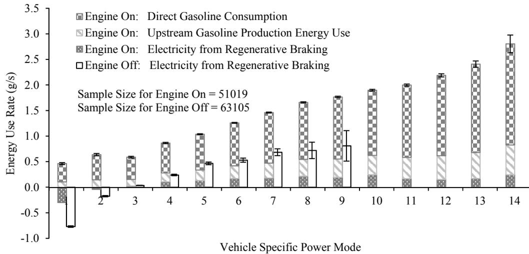
Figure S36 The Energy Use Rate Versus Vehicle Specific Power (VSP) Mode for Engine On and Off for Charge Sustaining (CS) Mode for a 2013 Toyota Prius Plug-In Hybrid Measured from January 18, 2013 to January 25, 2013 in Raleigh/Research Triangle Park, North Carolina Area
