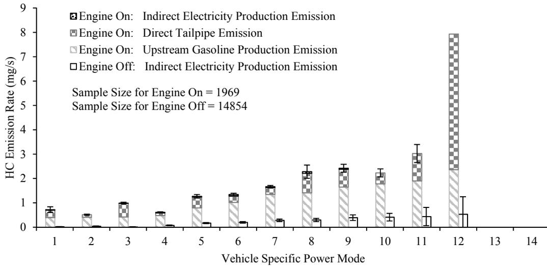
Figure S31 The Hydrocarbon (HC) Emission Rate Versus Vehicle Specific Power (VSP) Mode for Engine On and Off for Charge Depleting (CD) Mode for a 2013 Toyota Prius Plug-In Hybrid Measured from January 18, 2013 to January 25, 2013 in Raleigh/Research Triangle Park, North Carolina Area
