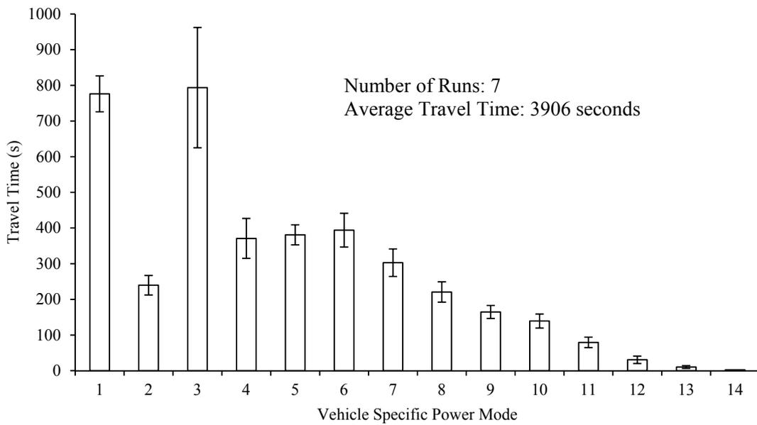
Figure S9 The Travel Time Distribution in Each Vehicle Specific Power Mode for Route 3
