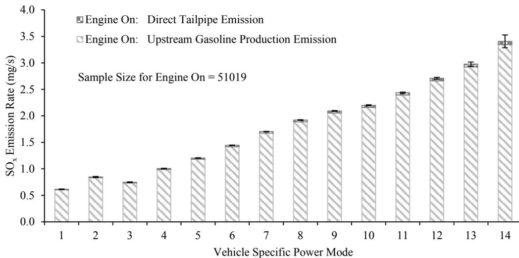
Figure S41 The Oxide of Sulfur (SO<sub>x</sub>) Emission Rate Versus Vehicle Specific Power (VSP) Mode for Engine On for Charge Sustaining (CS) Mode for a 2013 Toyota Prius Plug-In Hybrid Measured from January 18, 2013 to January 25, 2013 in Raleigh/Research Triangle Park, North Carolina Area
