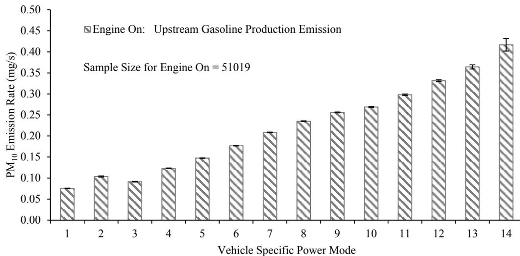
Figure S43 The Particulate Matter with Diameters of 10 Micrometers or Less (PM<sub>10</sub>) Emission Rate Versus Vehicle Specific Power (VSP) Mode for Engine On for Charge Sustaining (CS) Mode for a 2013 Toyota Prius Plug-In Hybrid Measured from January 18, 2013 to January 25, 2013 in Raleigh/Research Triangle Park, North Carolina Area
