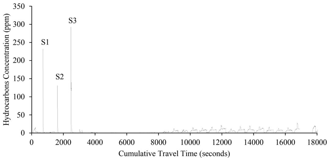
Figure S47 Second-by-Second the Hydrocarbons (HC) Concentration Data for a 2013 Toyota Prius Plug-In Hybrid Measured on January 21, 2013 in Raleigh/Research Triangle Park, NC Area
