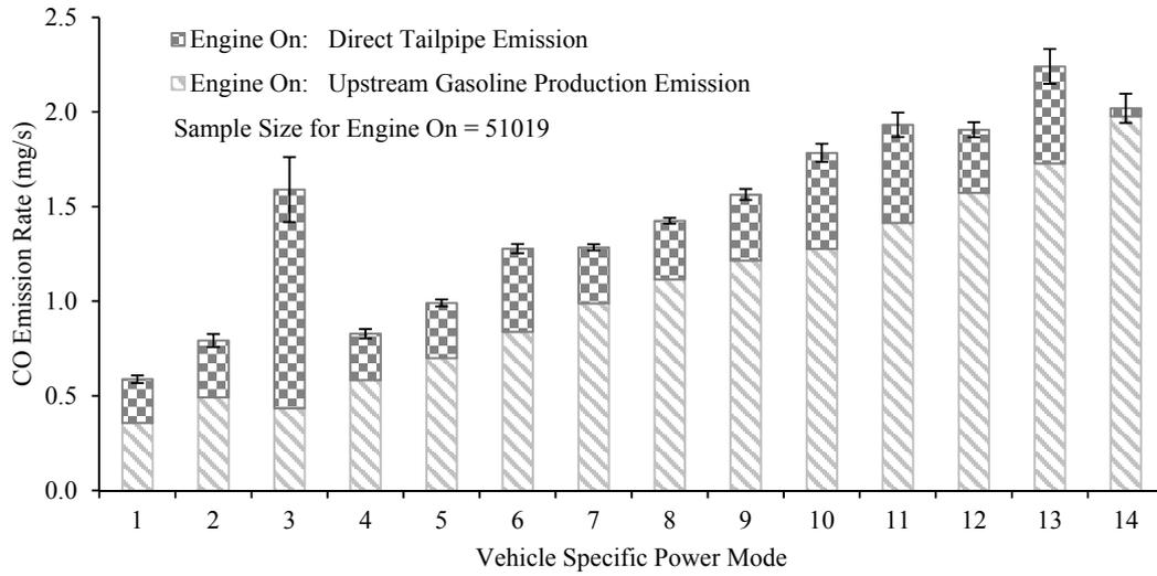
Figure S38 The Carbon Monoxide (CO) Emission Rate Versus Vehicle Specific Power (VSP) Mode for Engine On for Charge Sustaining (CS) Mode for a 2013 Toyota Prius Plug-In Hybrid Measured from January 18, 2013 to January 25, 2013 in Raleigh/Research Triangle Park, North Carolina Area
