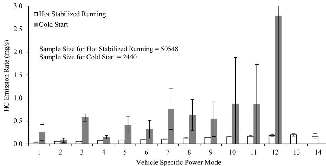
Figure S53 The Average Tailpipe Hydrocarbon (HC) Emission Rate Versus Vehicle Specific Power (VSP) Mode for Cold Start and Hot Stabilized Running During Engine On for a 2013 Toyota Prius Plug-In Hybrid Measured from January 18, 2013 to January 25, 2013 in Raleigh/Research Triangle Park, North Carolina Area
