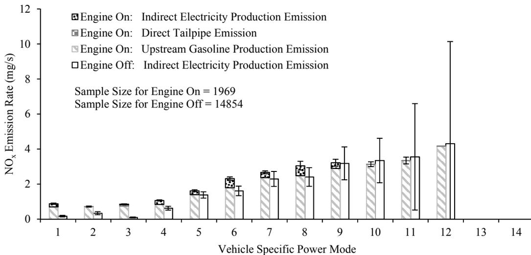
Figure S32 The Oxide of Nitrogen (NO<sub>x</sub>) Emission Rate Versus Vehicle Specific Power (VSP) Mode for Engine On and Off for Charge Depleting (CD) Mode for a 2013 Toyota Prius Plug-In Hybrid Measured from January 18, 2013 to January 25, 2013 in Raleigh/Research Triangle Park, North Carolina Area
