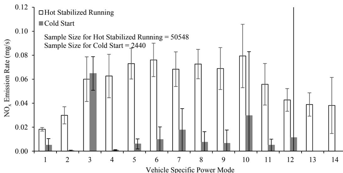
Figure S54 The Average Tailpipe Oxides of Nitrogen (NO<sub>x</sub>) Emission Rate Versus Vehicle Specific Power (VSP) Mode for Cold Start and Hot Stabilized Running During Engine On for a 2013 Toyota Prius Plug-In Hybrid Measured from January 18, 2013 to January 25, 2013 in Raleigh/Research Triangle Park, North Carolina Area
