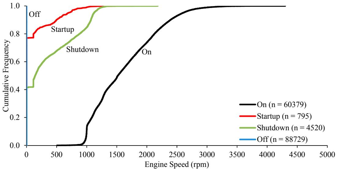
Figure S28 The Cumulative Distribution of Engine Speed for Engine “on”, “startup”, “shutdown”, and “off”, for All Vehicle Operation, Including Charge Depleting and Charge Sustaining Modes
