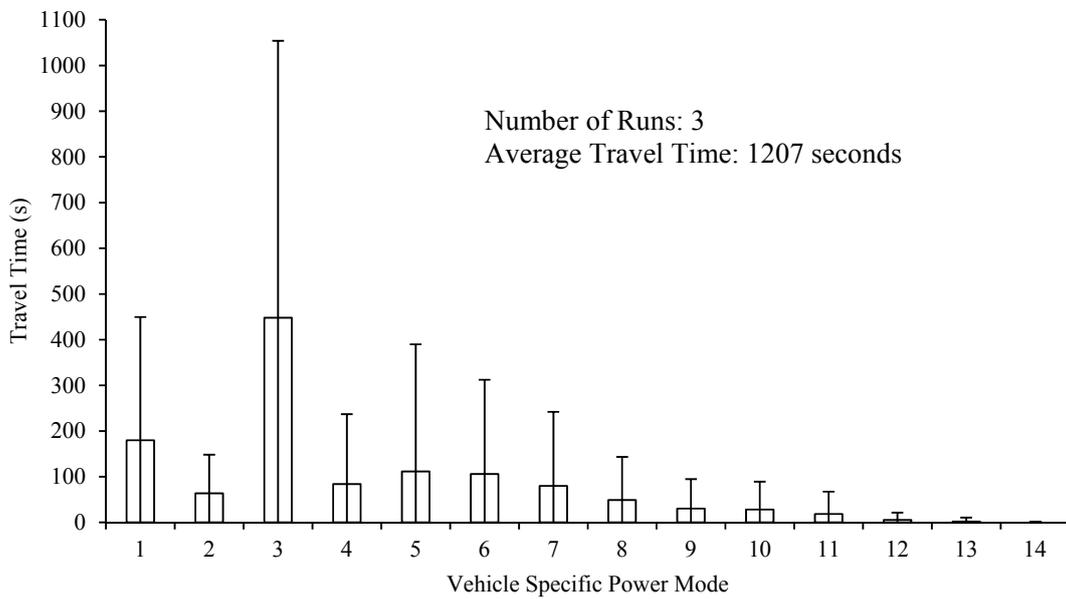
Figure S5 The Travel Time Distribution in Each Vehicle Specific Power Mode for Route D
