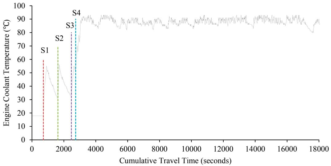
Figure S44 Second-by-Second the Engine Coolant Temperature Data for a 2013 Toyota Prius Plug-In Hybrid Measured on January 21, 2013 in Raleigh/Research Triangle Park, NC Area
