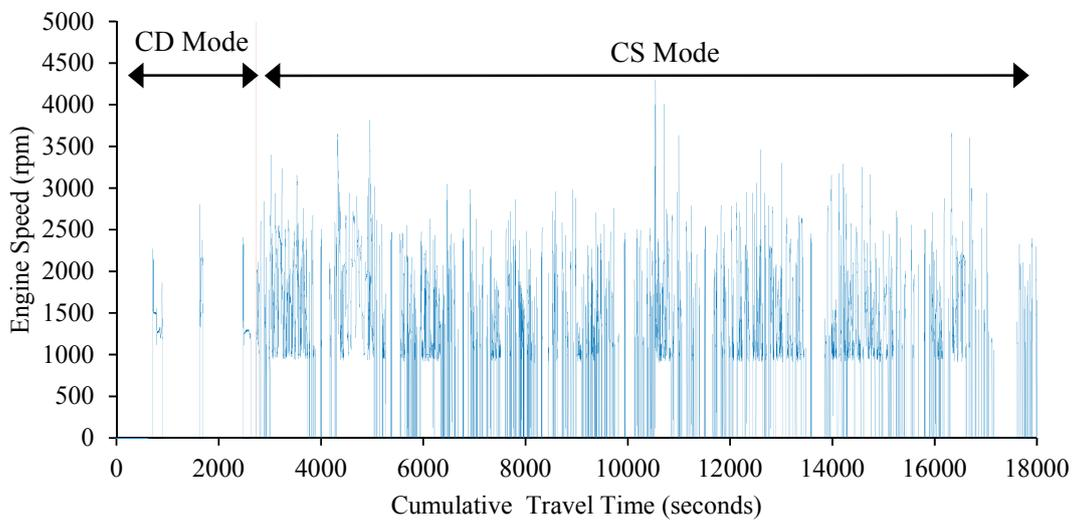
Figure S11 Second-by-Second the Engine Speed Data for Charge Depleting (CD) and Charge Sustaining (CS) Modes for a 2013 Toyota Prius Plug-In Hybrid Measured on January 21, 2013 in Raleigh/Research Triangle Park, NC Area
