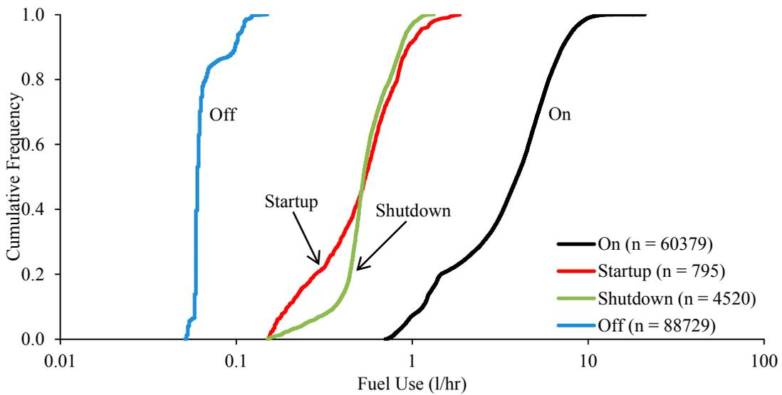
Figure S29 The Cumulative Distribution of Engine Fuel Use for Engine “on”, “startup”, “shutdown”, and “off”, for All Vehicle Operation, Including Charge Depleting and Charge Sustaining Modes
