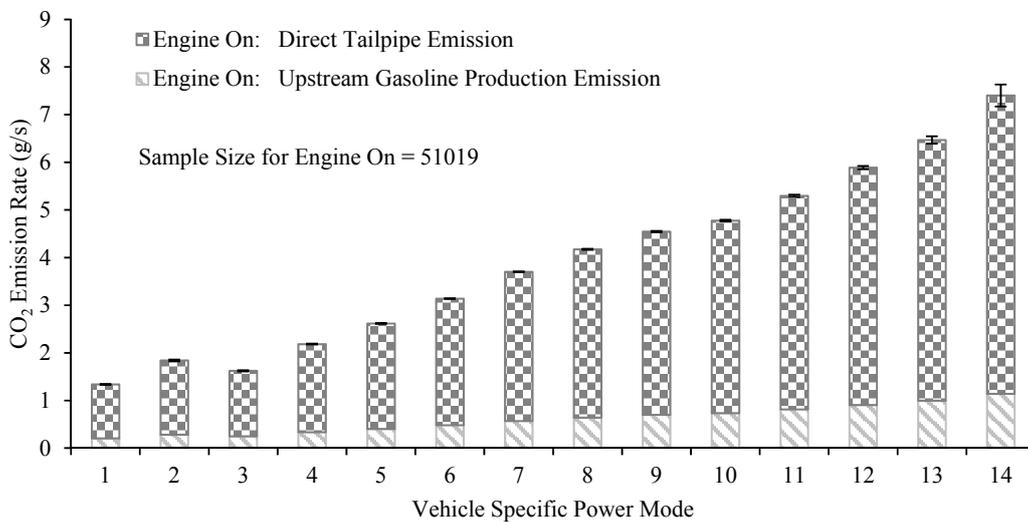
Figure S37 The Carbon Dioxide (CO<sub>2</sub>) Emission Rate Versus Vehicle Specific Power (VSP) Mode for Engine On for Charge Sustaining (CS) Mode for a 2013 Toyota Prius Plug-In Hybrid Measured from January 18, 2013 to January 25, 2013 in Raleigh/Research Triangle Park, North Carolina Area
