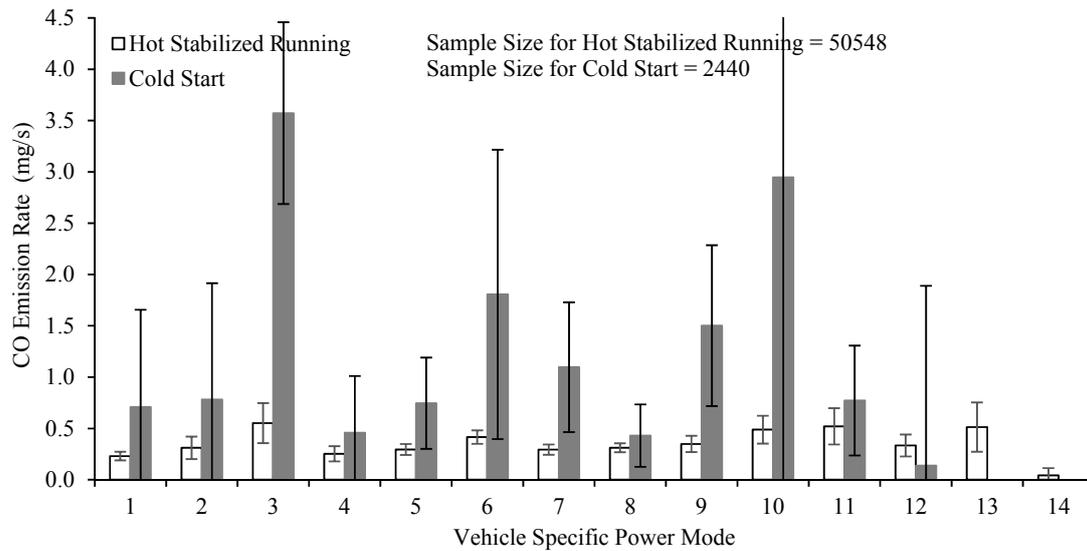
Figure S52 The Average Tailpipe Carbon Monoxide (CO) Emission Rate Versus Vehicle Specific Power (VSP) Mode for Cold Start and Hot Stabilized Running During Engine On for a 2013 Toyota Prius Plug-In Hybrid Measured from January 18, 2013 to January 25, 2013 in Raleigh/Research Triangle Park, North Carolina Area
