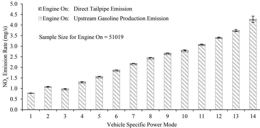
Figure S40 The Oxide of Nitrogen (NO<sub>x</sub>) Emission Rate Versus Vehicle Specific Power (VSP) Mode for Engine for Charge Sustaining (CS) Mode for a 2013 Toyota Prius Plug-In Hybrid Measured from January 18, 2013 to January 25, 2013 in Raleigh/Research Triangle Park, North Carolina Area
