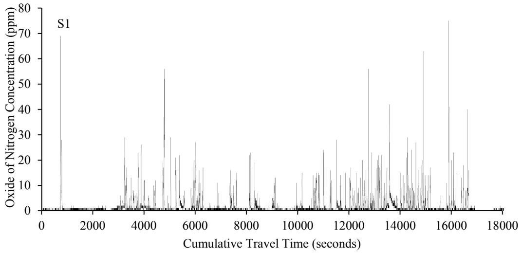
Figure S48 Second-by-Second the Oxide of Nitrogen (NO<sub>x</sub>) Concentration Data for a 2013 Toyota Prius Plug-In Hybrid Measured on January 21, 2013 in Raleigh/Research Triangle Park, NC Area
