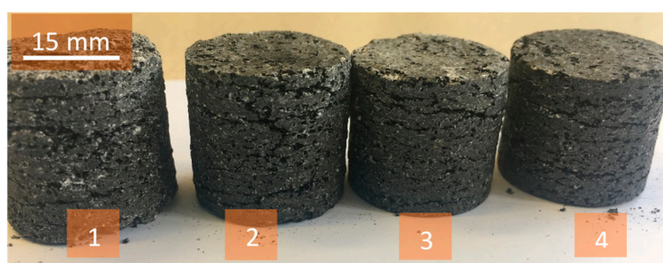
Figure 11. MSH/G+C pellet samples, No.1: MSH/G+C (0.4:1); No.2: MSH/G+C (0.6:1); No.3: MSH/G+C (0.8:1); No.4: MSH/G+C (1:1). All pellets were manufactured at a 5.2 \text{kN}\cdot\text{mm}^{-2} compression pressure.
