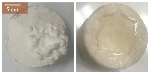
Figure 4. MSH pellet on the left and \text{SrBr}_2\cdot 6\text{H}_2\text{O} (SBH) pellets on the right after first dehydration test at 85 °C, 5% RH. Both pellets were manufactured under a 5.2 \text{ kN}\cdot\text{mm}^{-2} compression pressure.
