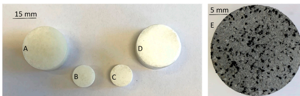
Figure 2. (A) A total of 10 g in mass of pure \text{SrBr}_2\cdot 6\text{H}_2\text{O} , 25 mm in diameter, 8.5 mm in thickness, and a 5.2 \text{ kN}\cdot\text{mm}^{-2} compression pressure. (B) A total of 0.3 g in mass of pure \text{SrBr}_2\cdot 6\text{H}_2\text{O} , 12 mm in diameter, 1.68 mm in thickness, and a 0.77 \text{ kN}\cdot\text{mm}^{-2} compression pressure. (C) A total of 0.3 g in mass of pure \text{MgSO}_4\cdot 7\text{H}_2\text{O} (MSH), 12 mm in diameter, 2.45 mm in thickness, and a 0.77 \text{ kN}\cdot\text{mm}^{-2} compression pressure. (D) A total of 10 g in mass of pure \text{MgSO}_4\cdot 7\text{H}_2\text{O} , 25 mm in diameter, 12.5 mm in thickness, and a 5.2 \text{ kN}\cdot\text{mm}^{-2} compression pressure. (E) MSH/G+C (1:1) composite pellet 10 g in mass, 25 mm in diameter, 9.8 mm in thickness, and a 5.2 \text{ kN}\cdot\text{mm}^{-2} compression pressure.
