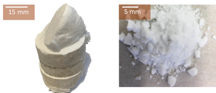
Figure 5. The structure of MSH pellets after four hydration/dehydration cyclic tests. Left: 25 mm diameter prepared under a compression pressure of 5.2 \text{ kN}\cdot\text{mm}^{-2} ; Right: 12 mm diameter prepared under a compression pressure of 0.77 \text{ kN}\cdot\text{mm}^{-2} .
