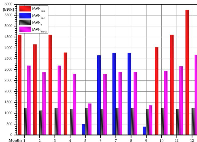
**Figure 3.** Allocation of the monthly energy consumption of the building for a typical year.
