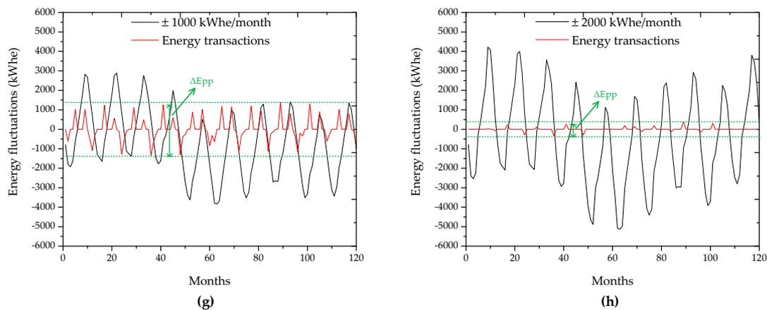
**Figure 7.** Monthly energy fluctuations in the EESU and energy transactions with the electricity grid for each scenario of EESU maximum permitted storage energy fluctuations. Maximum Permitted EESU Energy Fluctuations Per Month (kWh<sub>e</sub>/month: (a) 0, (b) ±100, (c) ±250, (d) ±400, (e) ±500, (f) ±750, (g) ±1000, (h) ±2000.
