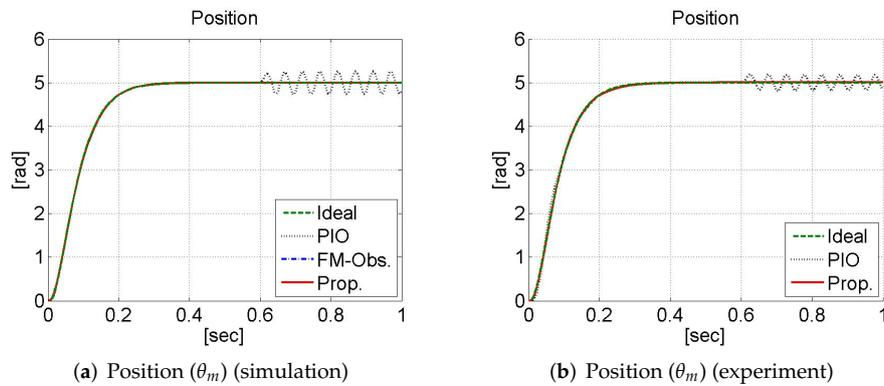
Figure 4. Results of DC motor position.
