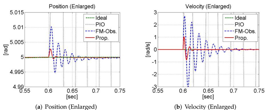
Figure 6. Results of DC motor position (enlarged).
