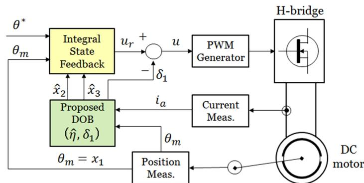
Figure 3. Control block of DC motor control system.
