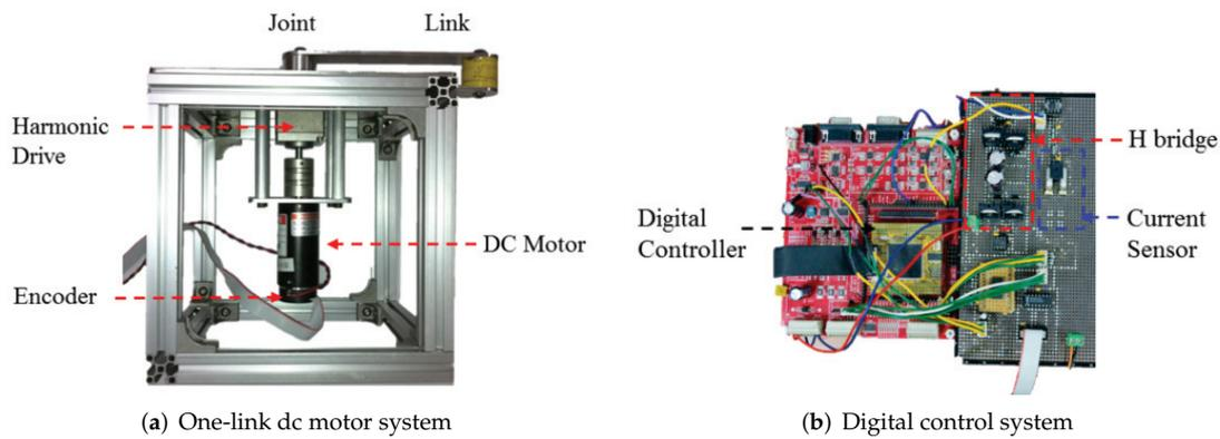
**Figure 2.** DC motor control system for experimental tests.
