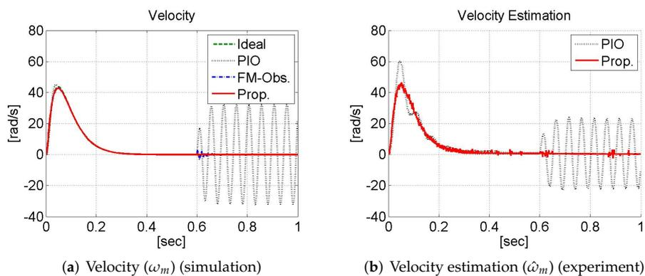
Figure 5. Results of DC motor velocity.
