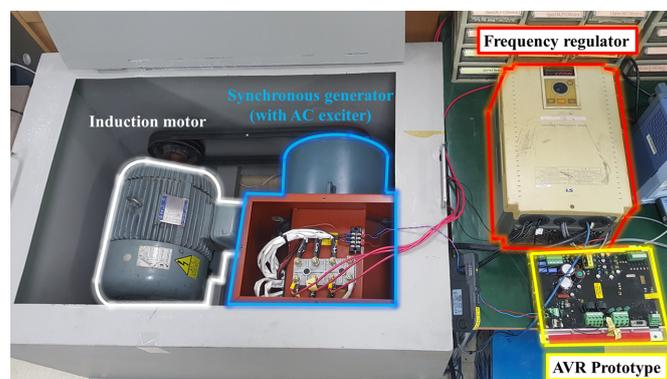
**Figure 22.** Motor-generator set for imitation of the speed regulator in a synchronous generator system.
