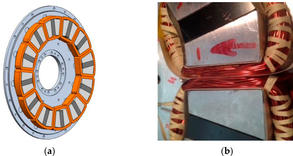
Figure 1. (a) Demonstration of the stator windings; (b) photo of the windings of the prototype.
