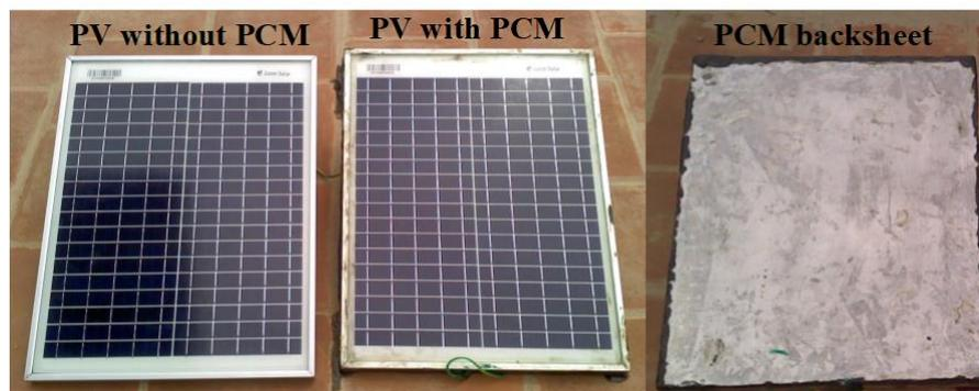
**Figure 1.** Experimental setup for PV with and without PCM using OM29.
