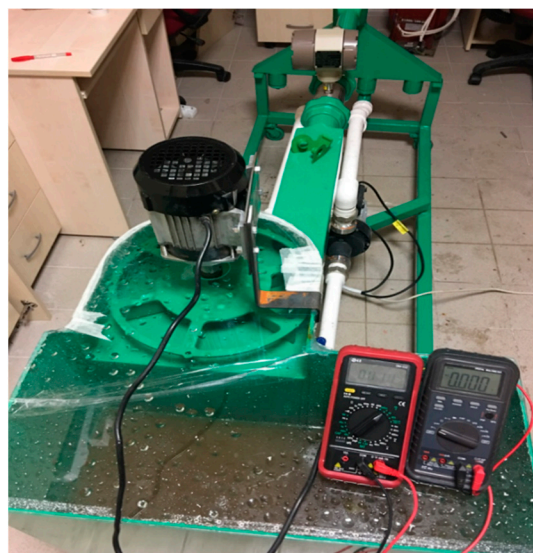
Figure 2. Experimental setup of vertical hydrokinetic turbine.
