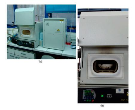
**Figure 1.** Experimental setup of the torrefaction process: (**a**) Nuve Muffle Furnace (Internal dimensions:  $210W \times 300D \times 110$ Hmm) equipped with electric heating and a nitrogen generator that uses molecular sieves and (**b**) barley straw in a ceramic crucible placed in the cold furnace.
