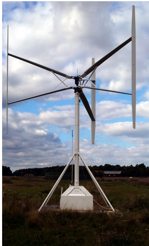
Figure 3. The 12 kW turbine, designed and built by the Division of Electricity at Uppsala University. The turbine is equipped with load cells used for the force measurements [21].
