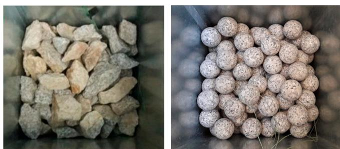
**Figure 4.** Crushed rock and spheres arranged inside the bed storage.
