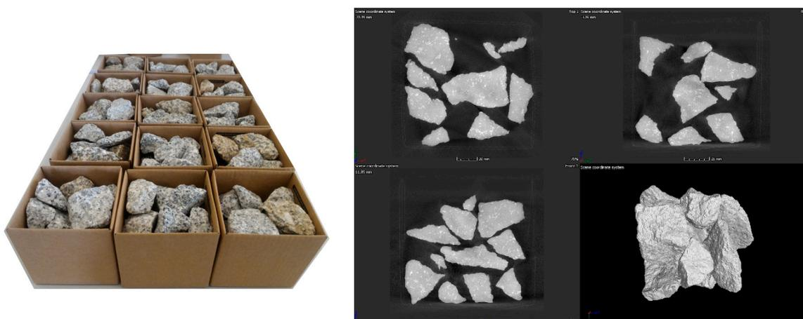
**Figure 1.** Material prepared for tomographic examination and exemplary scans of the granite crushed rock.
