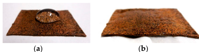
Figure A2. Images of MCF rubber before and after water permeation (0.75 g of MF, 0.5 g of TiO 2 , 3 g of S-500, 3 g of 671A, and 3 g of Ni): (a) before permeation; (b) after permeation [41].
