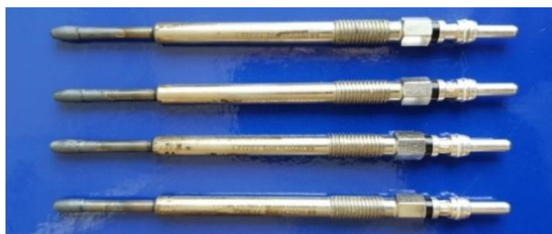
Figure 5. Glow plug with the catalytic layer (heating part—30 mm).
