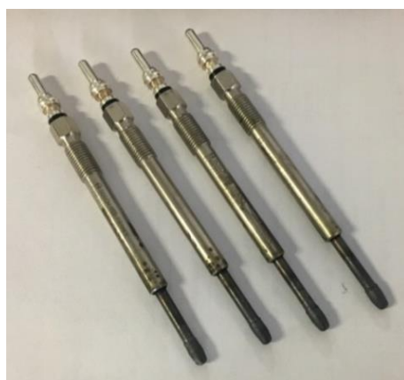
Figure 6. Prototype glow plugs with the elongated heating part (34 mm).
