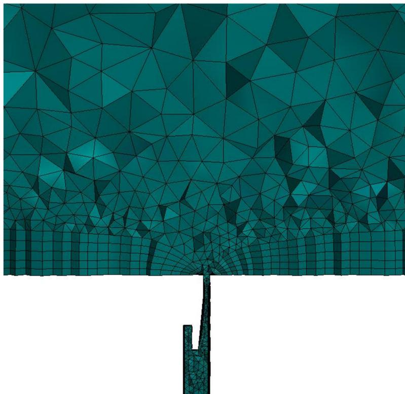
**Figure 3.** Close up to the jet's outlet cross-section volume mesh.
