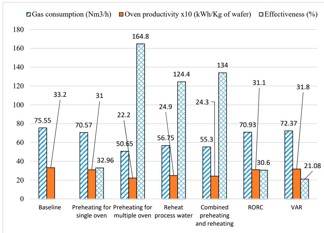
**Figure 11.** Comparison of heat recovery technologies based on oven’s gas consumption, productivity and effectiveness. Note: the oven productivity values have been multiplied by 10 to fit the graph.
