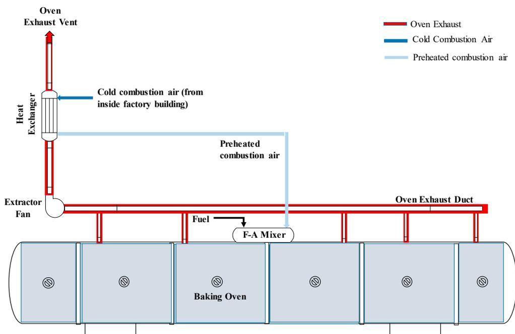
**Figure 3.** Schematic of combustion air preheating process using oven exhaust.
