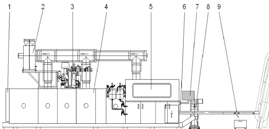
**Figure 1.** Schematic of a pilot-scale wafer baking oven highlighting the key components of the oven [37].
