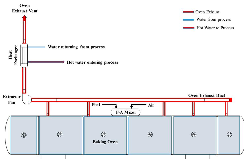
**Figure 4.** Schematic of the heating returning process water using oven exhaust.
