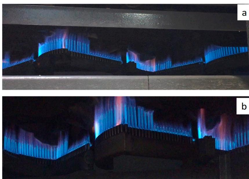
**Figure 8.** Flame colour before (a) and after (b) combustion air preheating.
