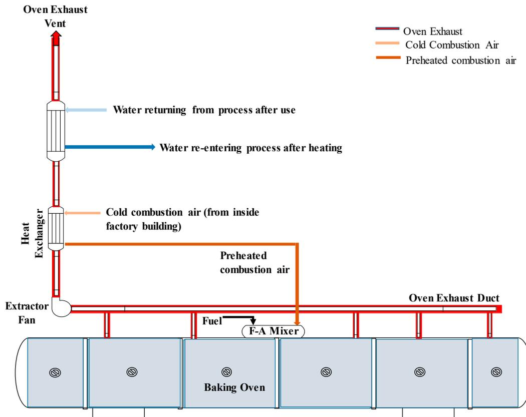
**Figure 9.** Schematic of combustion air preheating combined with reheating process water using oven exhaust gases.
