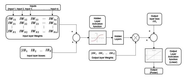
Figure 3. Vector-matrix notation based structural representation of ANN.
