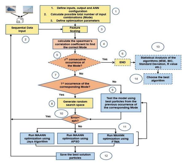
**Figure 6.** Flow chart for the dynamic learning algorithm for renewable energy sources power generation prediction.
