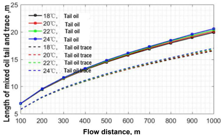
Figure S26. Effect of temperature on the length of tail and trail part of mixed oil
