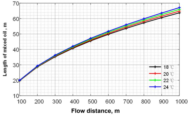
Figure S24. Effect of temperature on the length of mixed oil
