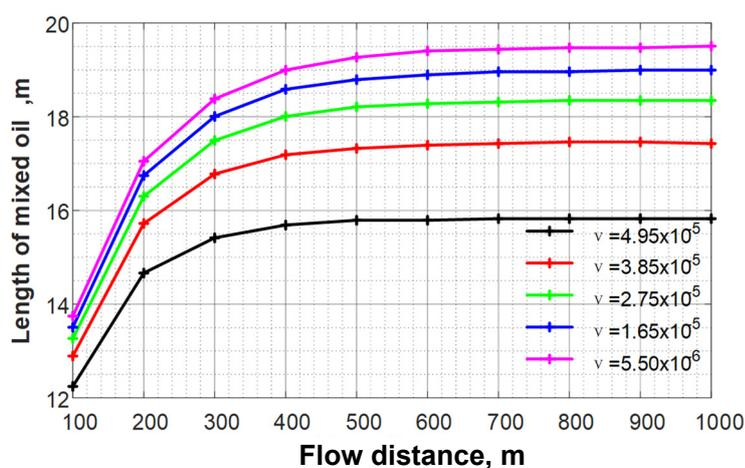
Figure S11. Effect of viscosity on the length of mixed oil
