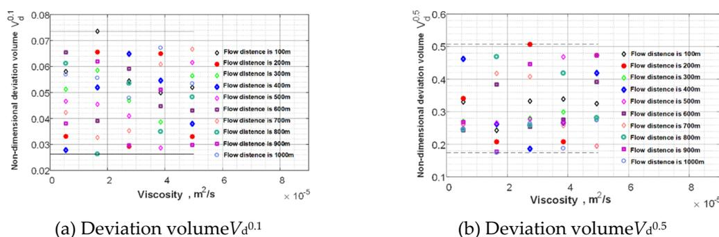
Figure S16. Effect of viscosity on deviation volume
