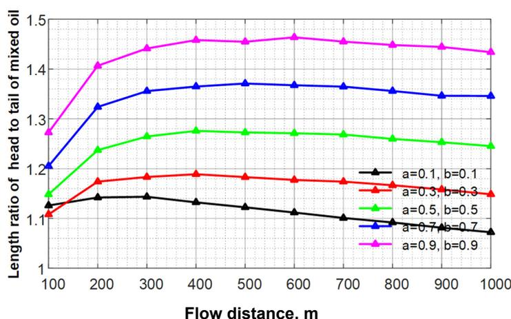
Figure S5. Effect of coefficient  $a$  and  $b$  to the ratio of front length and tail length
