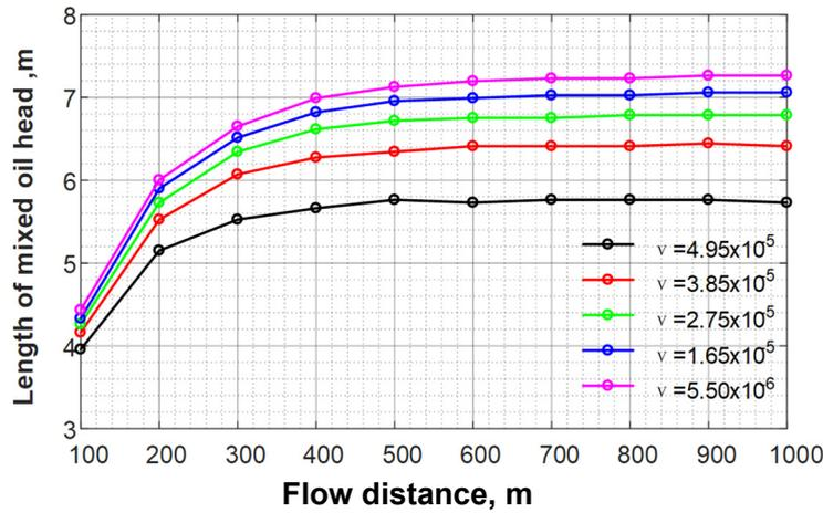
Figure S12. Effect of viscosity on front part of mixed oil
