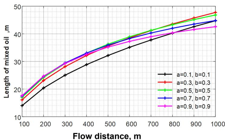
Figure S1. Effect of adsorption and desorption coefficient  $a$  and  $b$  to the length of mixed oil
