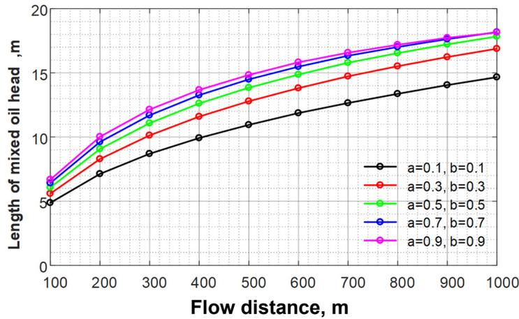
**Figure S2.** Effect of adsorption and desorption coefficient  $a$  and  $b$  to the length of front part of mixed oil
