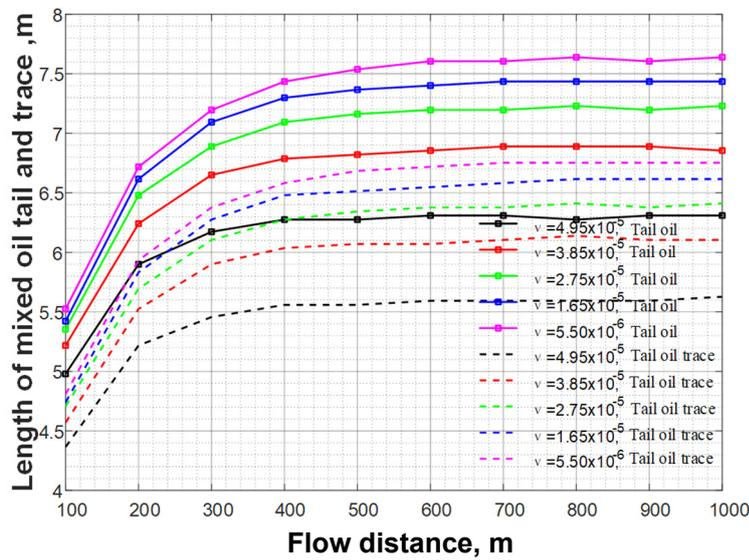
Figure S13. Effect of viscosity on tail and tail part of mixed oil
