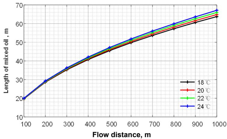
Figure S25. Effect of temperature on front part
