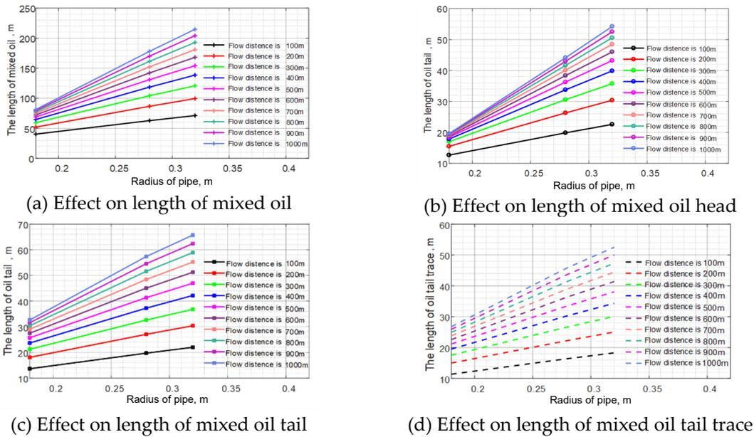
Figure S36. Effect of radius on the length of mixed oil, front part, tail part and trail part of mixed oil
