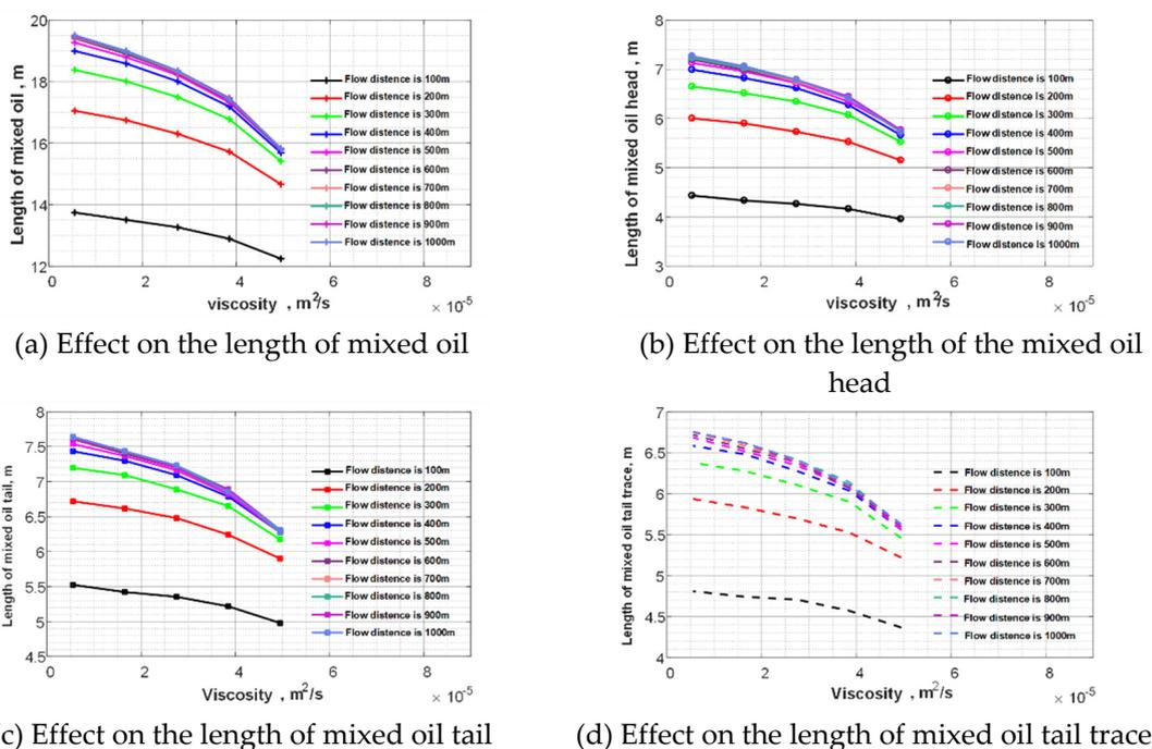
Figure S15. Effect of viscosity to length of mixed oil, front part, tail part and trail part of mixed oil
