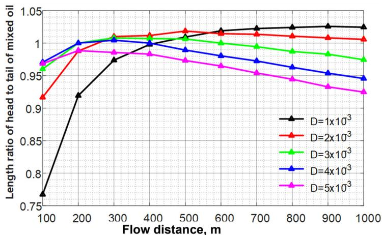
Figure S21. Ratio of front length and tail length changing with time for different D Diffusion coefficient distribution
