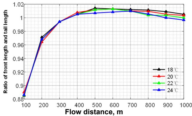
Figure S28. Ratio of front length and tail length changing with time for different temperature
