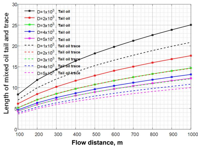
Figure S19. Effect of D on the length of tail and trail part of mixed oil
