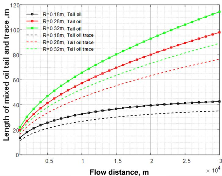
Figure S33. Effect of radius on the length of tail and trail part of mixed oil
