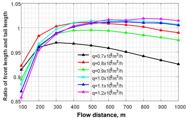
Figure S42. Ratio of front length and tail length changing with time for different velocity
