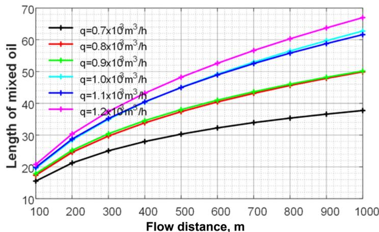
Figure S38. Effect of velocity on the length of mixed oil
