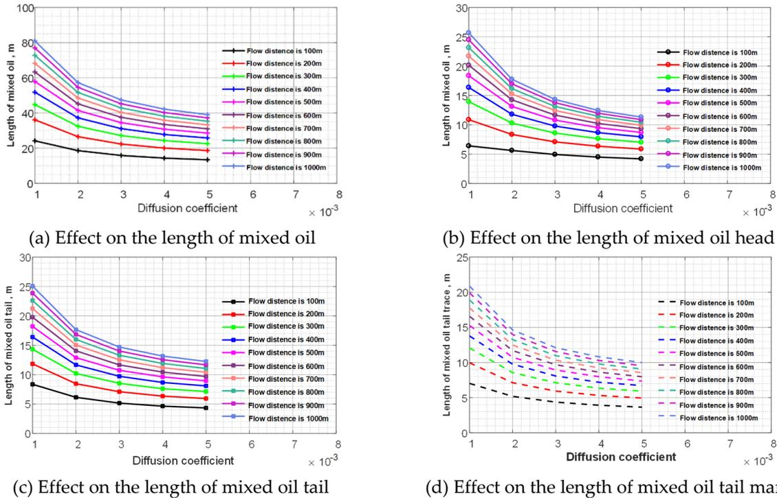
**Figure S22.** Effect of D on length of mixed oil, front part, tail part and trail part of mixed oil
