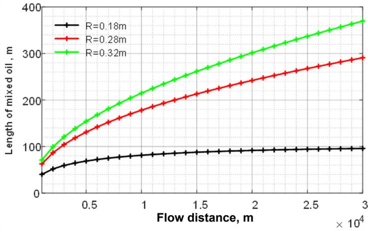
Figure S31. Effect of radius on the length of mixed oil
