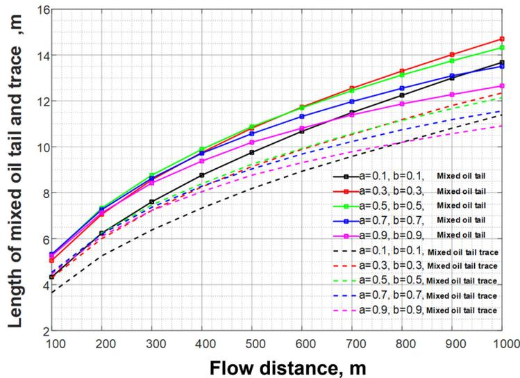
**Figure S3.** Effect of coefficient  $a$  and  $b$  to the length of tail and trail part of mixed oil
