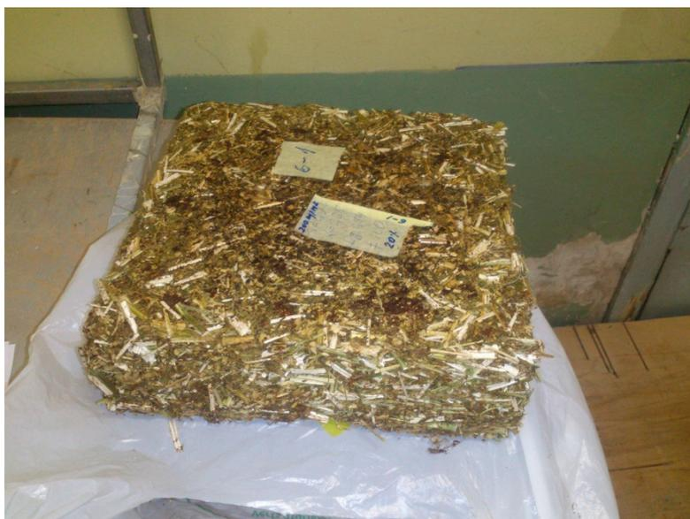
**Figure 2.** Slabs of hemp fibers with dimensions of 300 × 300 mm.
