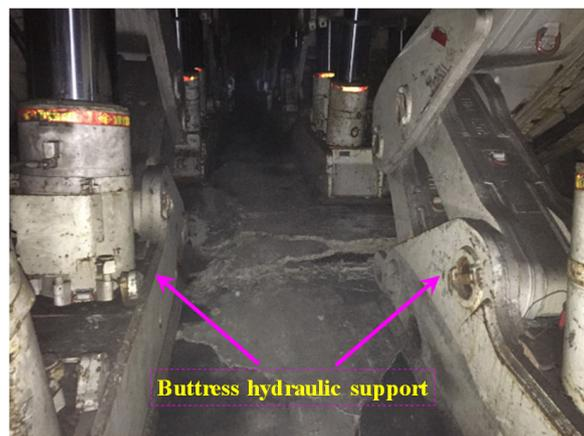
Figure 15. Photos of buttress hydraulic supports on site.
