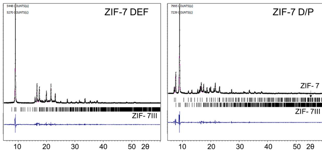
**Figure S2.** Powder XRD patterns of samples of ZIF-7 DEF (left one) and ZIF-7 D/P (right one): observed (black), calculated (magenta), and their difference (dark blue). The short vertical bars indicate the Bragg positions of the reflections (obtained using the Jana2006 program package).
