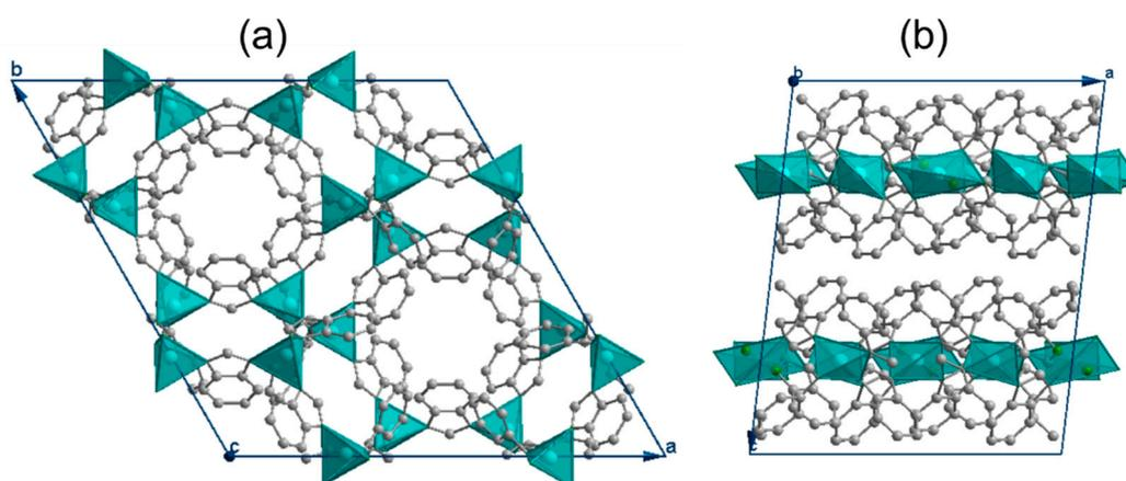
**Figure S1.** Schematic representation of ZIF-7 (a) and ZIF-7 III (b) unit cells. Blue tetrahedra represent Zn coordination with nitrogen atoms and gray-carbon atoms. Crystallographic axes are provided on the cell edges.
