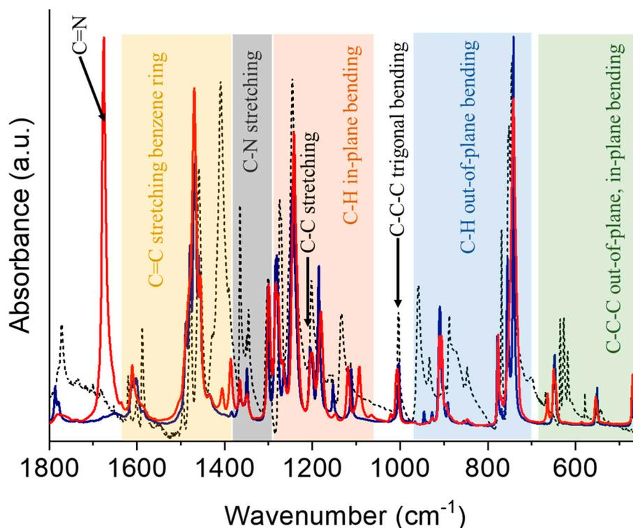
**Figure S6.** FTIR-spectra of samples ZIF-7 DEF (dark blue, ZIF-7 III phase) and ZIF- DMF (red, ZIF-7 phase).
