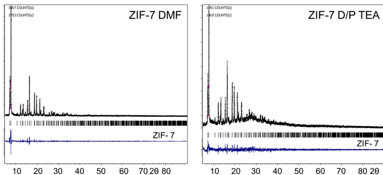
**Figure S3.** Powder XRD patterns of samples of ZIF-7 DMF (left one) and ZIF-7 D/P TEA (right one): observed (black), calculated (magenta), and their difference (dark blue). The short vertical bars indicate the Bragg positions of the reflections (obtained using the Jana2006 program package).
