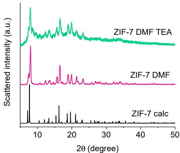
**Figure S4.** Powder XRD patterns of samples ZIF-7 DMF (pink one) and ZIF-7 DMF TEA (green one). Powder profile ZIF-7 calc was calculated according to crystallographic data (COD ID 412899).
