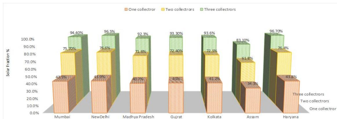
Figure 15. Solar fraction for evacuated collectors.
