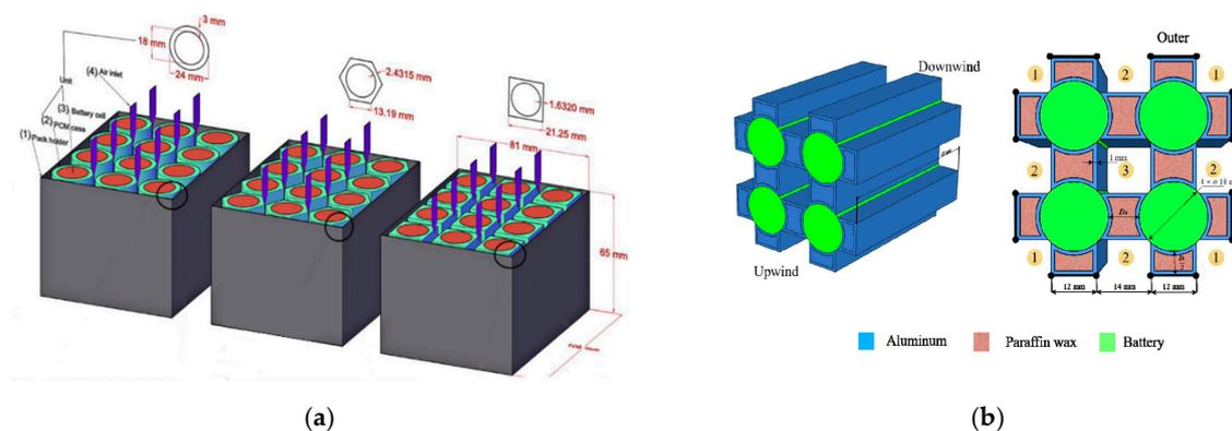
**Figure 7.** The geometry in PCM-based hybrid BTMS (a) Three different shapes of the cross section for PCM-based BTMS Reprint with permission [68]; 2020, Elsevier.; (b) Schematic of a PCM-based BTMS. Reprint with permission [69]; 2020, Elsevier.
