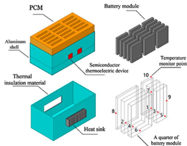
**Figure 10.** A classic example of hybrid BTMS of PCM coupled with TEC. Reprint with permission [77]; 2020, Elsevier.
