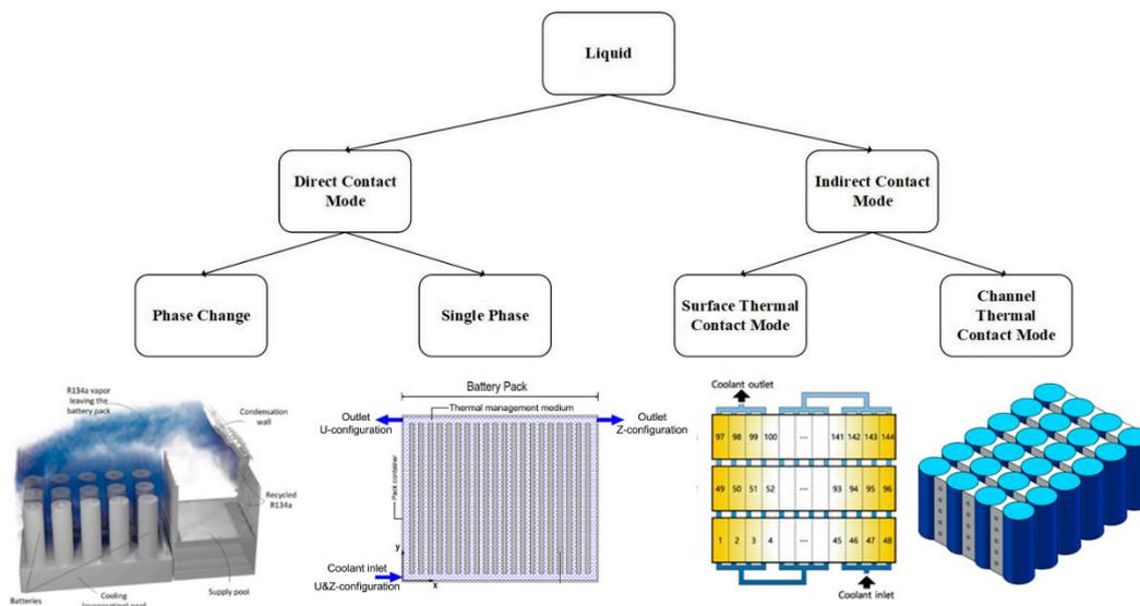
Figure 3. Classification of liquid cooling and corresponding classic examples [40–43].
