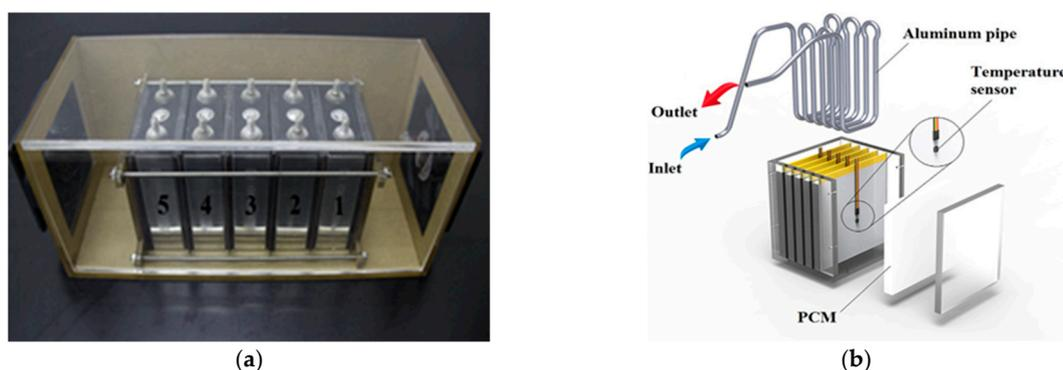
**Figure 5.** Examples for PCM-based hybrid BTMS (a) PCM+Air. Reprint with permission [57]; 2020, Elsevier., (b) PCM+Liquid. Reprint with permission [58]; 2020, Elsevier.
