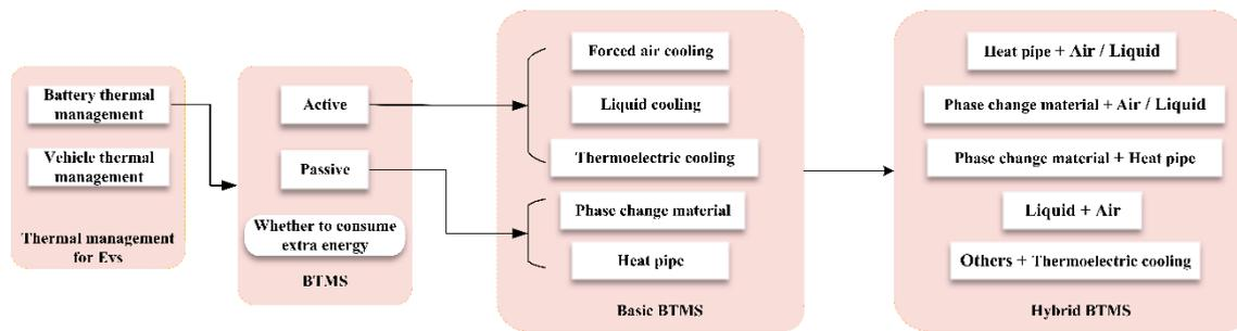
Figure 1. Classification of battery thermal management systems (BTMS).
