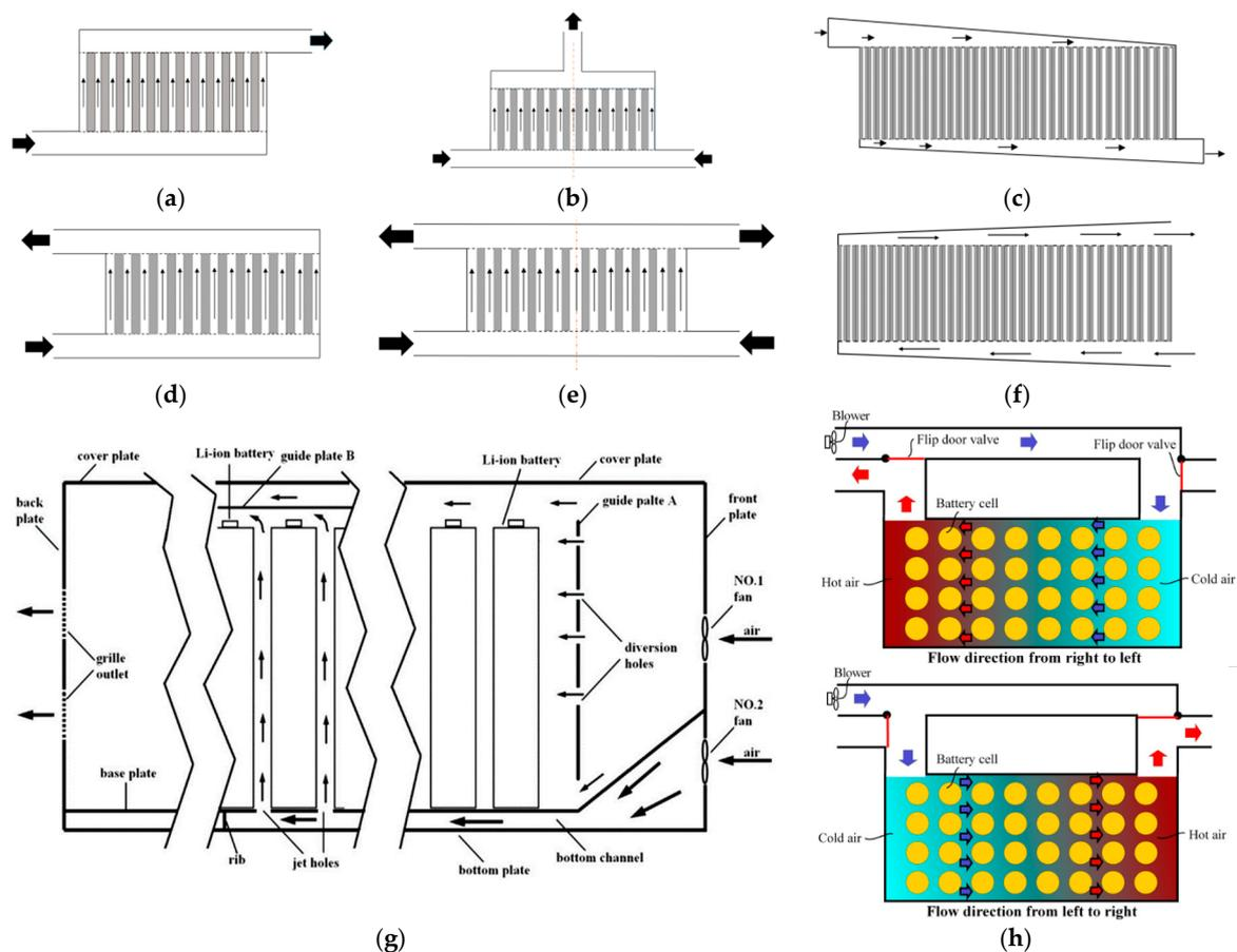
**Figure 2.** Designs of the flow channel and flow pattern (a,b,d,e) “Z-type” flow channel, Symmetrically modified “Z-type”, “U-type” flow channel, Symmetrically modified “U-type” [1], (c) Tapered “Z-type” [2], (f) Tapered “U-type”, (g) Additional duct, Reprint with permission [34]; 2020, Elsevier. (h) Reciprocating air flow in two directions. Reprint with permission [35]; 2020, Elsevier.
