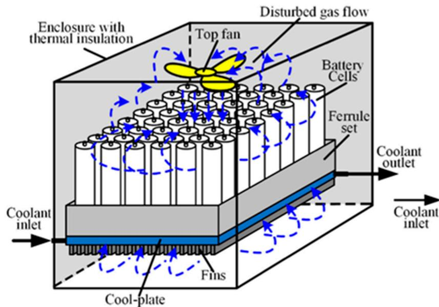
**Figure 11.** A classic example of BTMS based on liquid coupled with air. Reprint with permission [79]; 2020, Elsevier.
