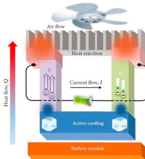
**Figure 9.** The schematic diagram of TEC in hybrid BTMS [78].
