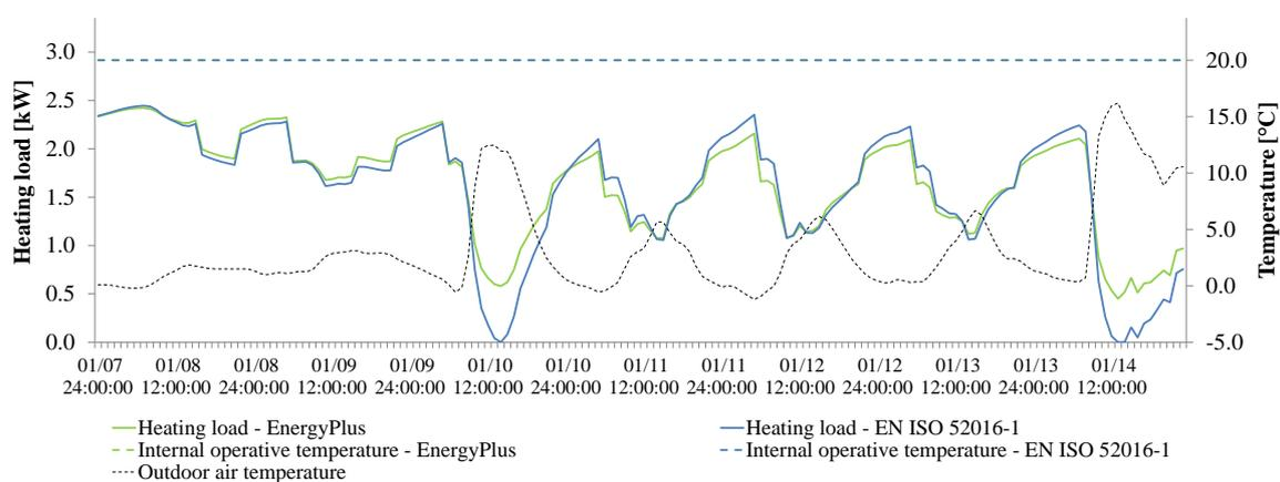
Figure 6. Heating loads for a week of January.
