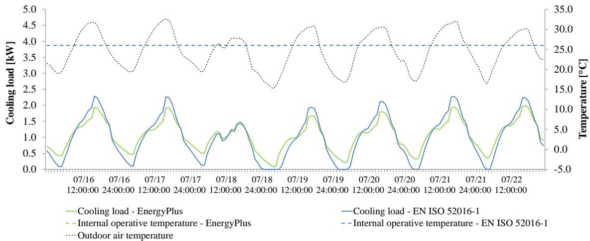
Figure 7. Cooling loads for a week of July.
