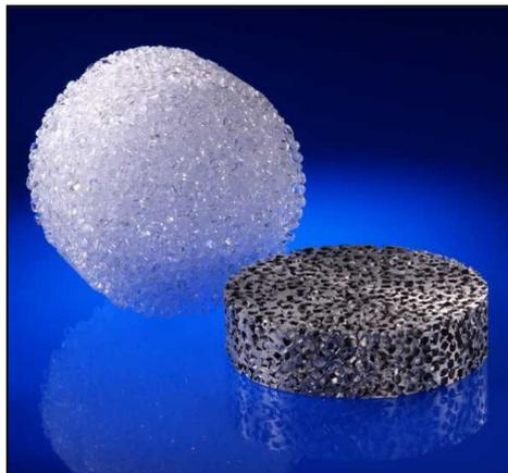
**Figure 1.** Polymer preform (left) and open porous aluminum foam (right).
