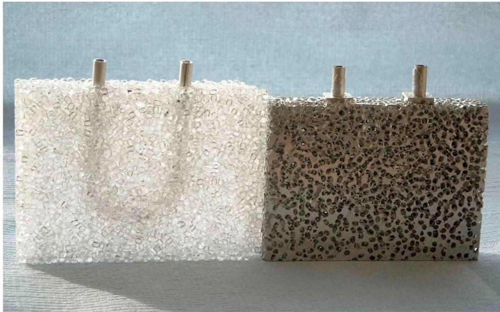
**Figure 2.** Polymer preforms (left) and open porous aluminum foams (right) with embedded tubes, for the 26p-system.
