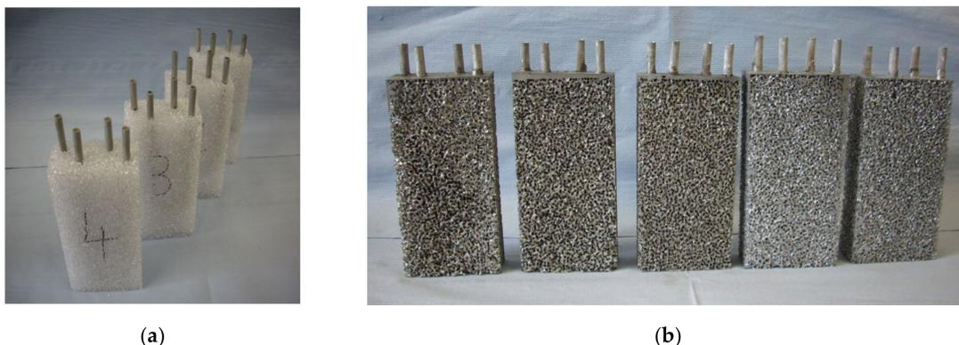
**Figure 3.** Polymer preforms (a) and open porous aluminum foams (b) with embedded tubes, for the 4p-system.
