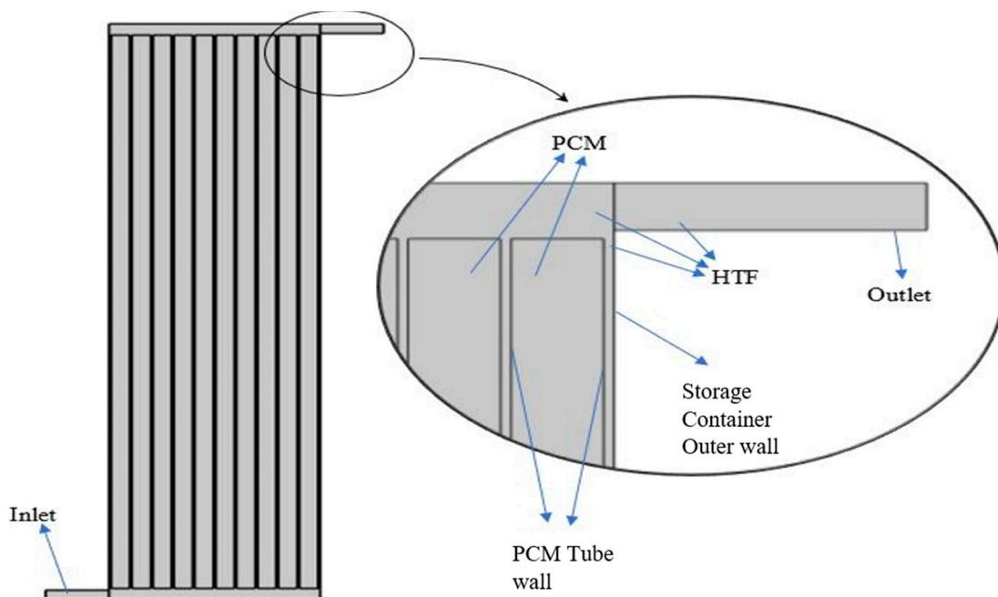
**Figure 1.** Energy storage tank modeling in COMSOL.
