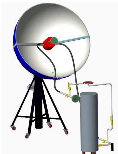
**Figure 6.** CAD/CAM Model of the solar concentrator.
