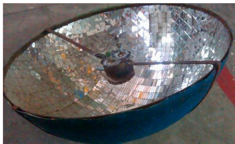
**Figure 7.** Manufactured solar concentrator.
