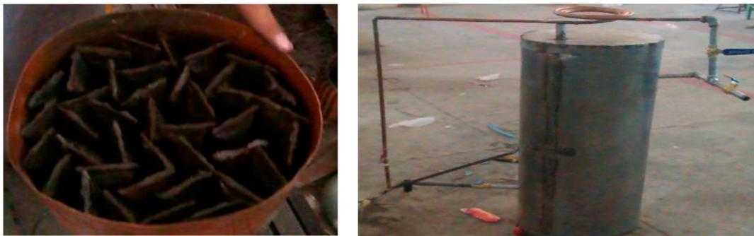
Figure 9. Fabrication of the storage tank.
