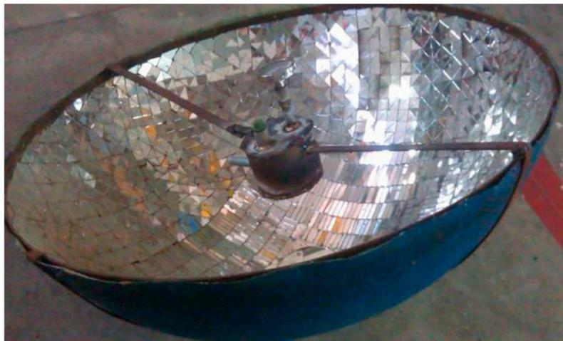
**Figure 7.** Manufactured solar concentrator.
