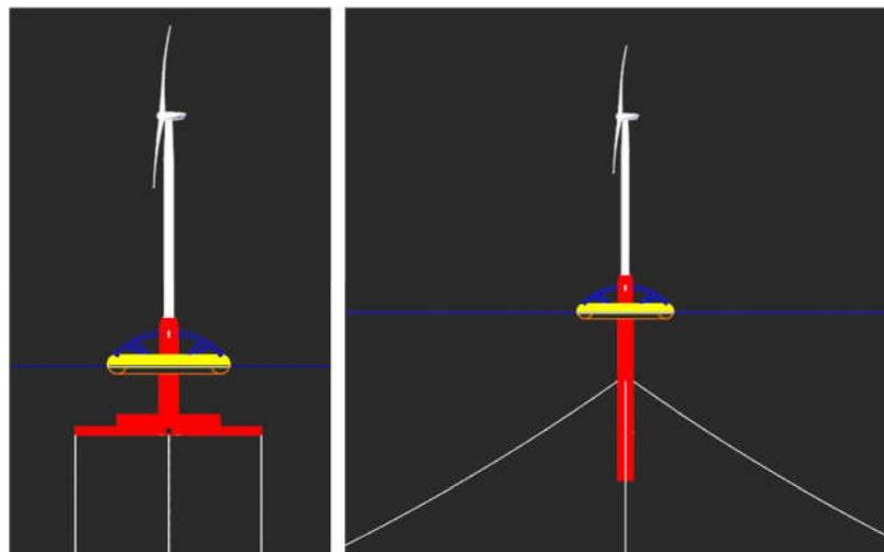
**Figure 1.** Conceived hybrid wind-wave energy system (HWWES): Wave energy converter (WEC) coupled with the TLP type platform (left); WEC coupled with SB type platform (right).
