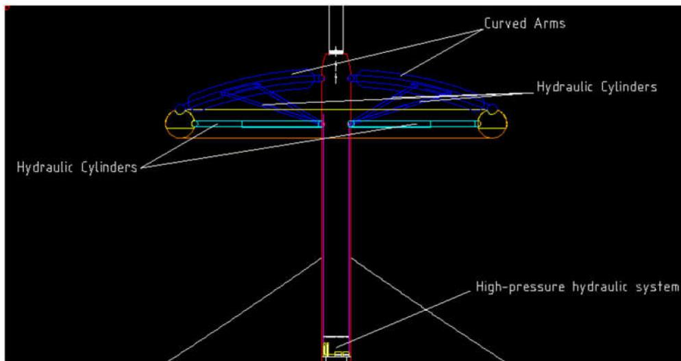
Figure 2. HWWES: WEC cross-section.
